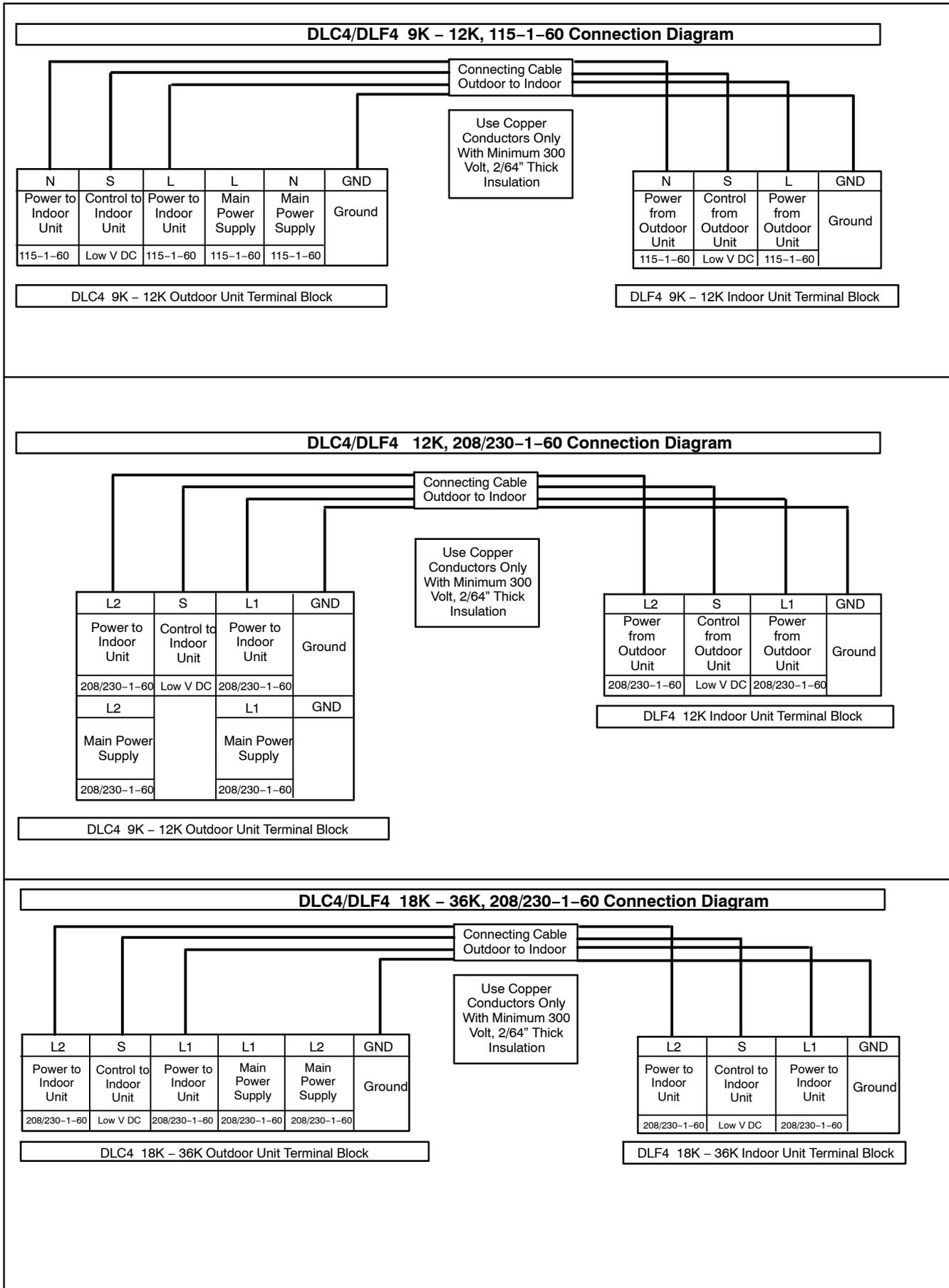
Figure 7 – Connection Diagrams
