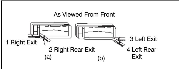
**Figure 10 – Refrigerant Line Routing**
