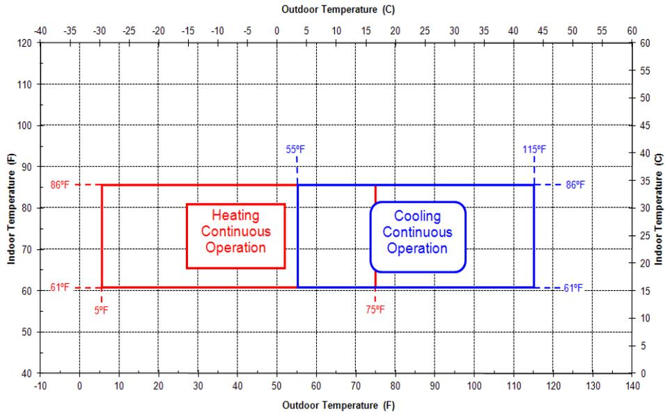
**Figure 3 – 9k / 12k 115V System Operating Envelopes**
