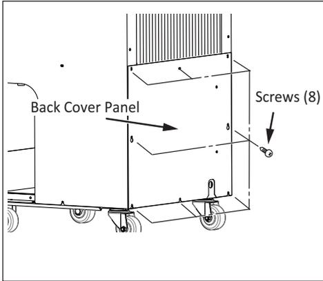
10) Take out the eight (8) screws, and then remove the back cover panel.
