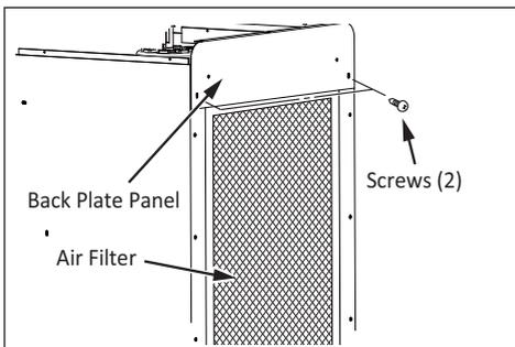
8) Remove the air filter from the back panel.
