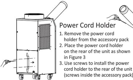
Figure 3 – Power Cord Holder attachment
