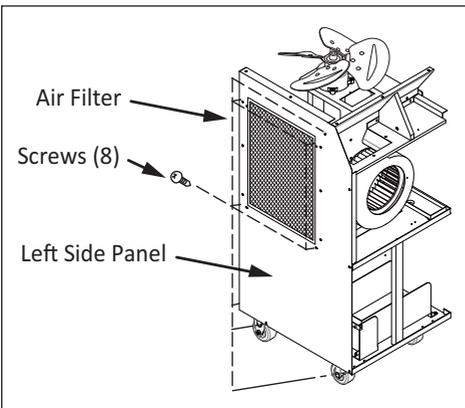
11) Remove the air filter from the left-side panel.
