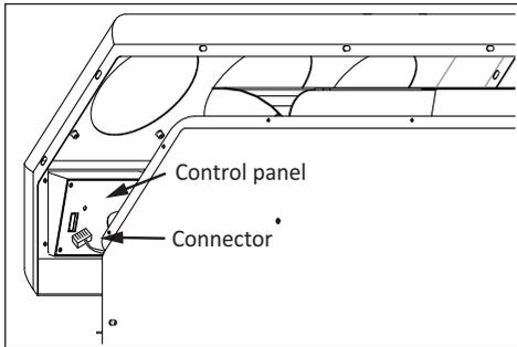
7) Unfasten the connector from the control panel and then remove the front panel.
