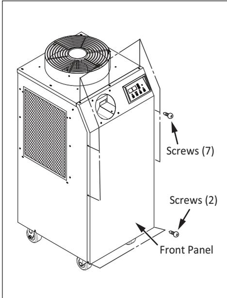
5) Take out the seven (7) screws. Unfasten two (2) screws to a half point. Pull the front panel forward.
