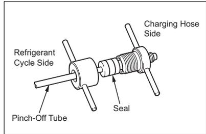
**NOTE:** Connect the hoses using care not to mistake the high pressure side for the low pressure side and vice versa.
