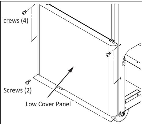
10) Take out the four (4) screws. Unfasten two (2) screws to a half point and then remove the low cover panel.
