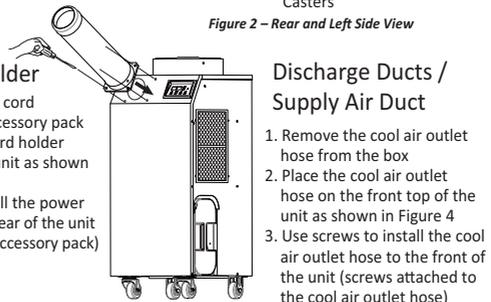
Figure 4 – Cool Air Outlet attachment
