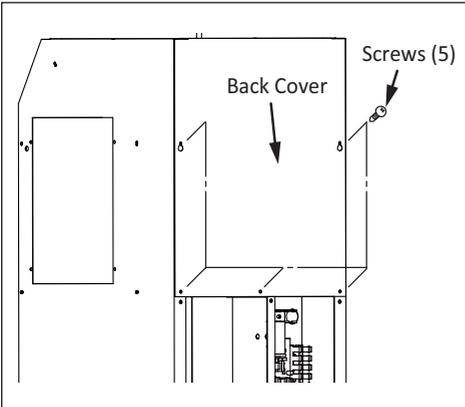
8) Take out the five (5) screws, and then remove the back cover.
