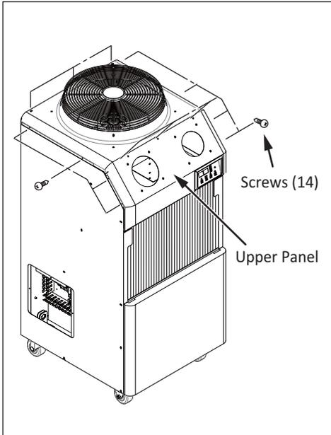
6) Take out the fourteen (14) screws, and then remove the upper panel.
