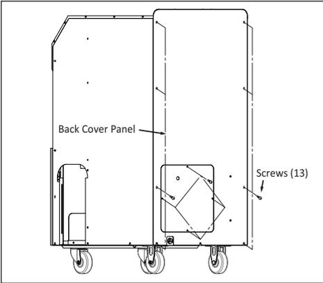
9) Take out the thirteen (13) screws, and then remove the back cover panel.
