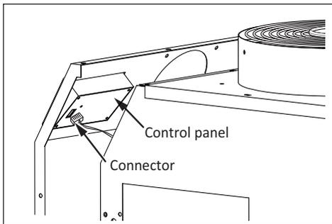
6) Disconnect the connector from the control panel and then remove the front panel.
