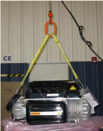
Figure 8 Rigging Set-up
