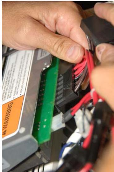
**Figure 4 Connect Test Harness to Soft-Start Board (As Seen From Top Side of Board)**
