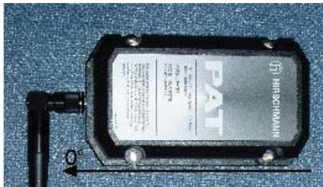
Angle sensor, transmitter, and mounting plate.
