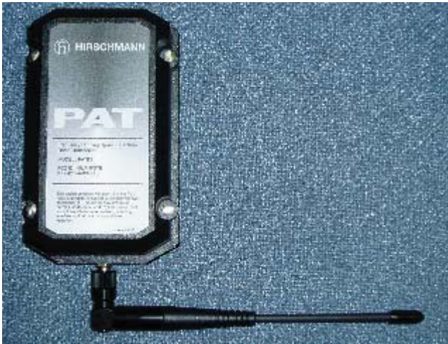
Angle sensor with transmitter 031-300-060-592
