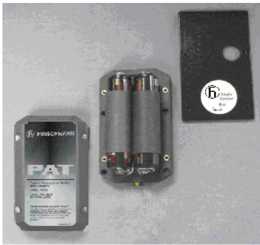
Angle sensor, transmitter, and mounting plate.
