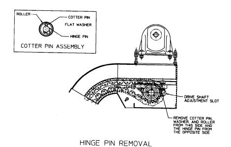
9. Grasp the end of belt below the drive shaft and pull the belt out of the conveyor. Be sure to wear gloves to avoid being cut by sharp edges on the belt. When only a few feet of belt remain in the conveyor, the belt on
