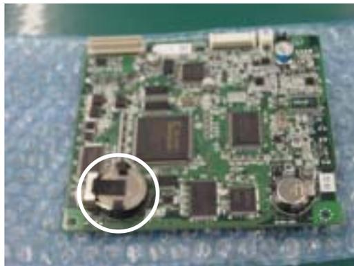
2. After the battery replacement, check the continuity between the battery terminal and receptacle terminal with a multimeter or digital voltmeter.
