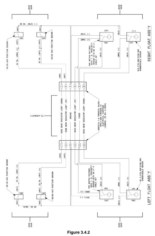
General wiring schematic for Float and Sensor layout
