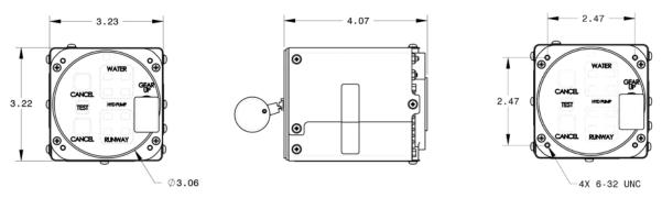
Figure 1.5.1 Housing and Mounting Hole Dimensions
