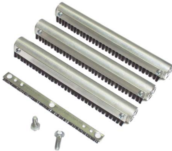
Fig. 8 The antistatic kit consists of brushes, which create a leading contact between label material or ribbon and the printer.
