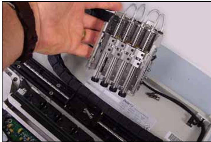
Figure U-37—The PNP Head Partially Removed
