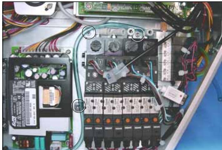
Figure U-16—Pneumatic Module fastener locations. The Probe Vacuum Tubes have been Disconnected.
