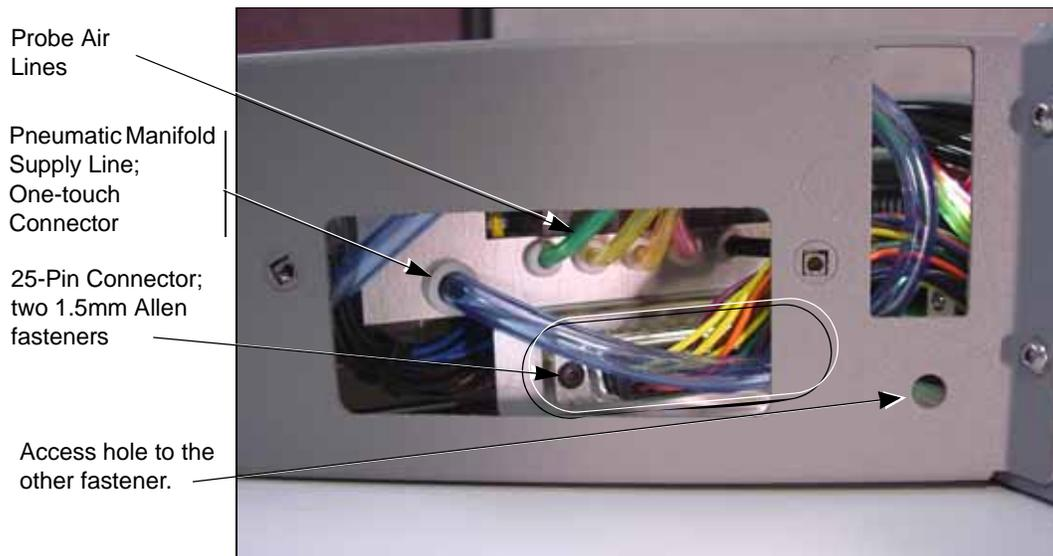
Figure U-15—Location of the Pneumatic Manifold Supply Line and Wiring Connector
