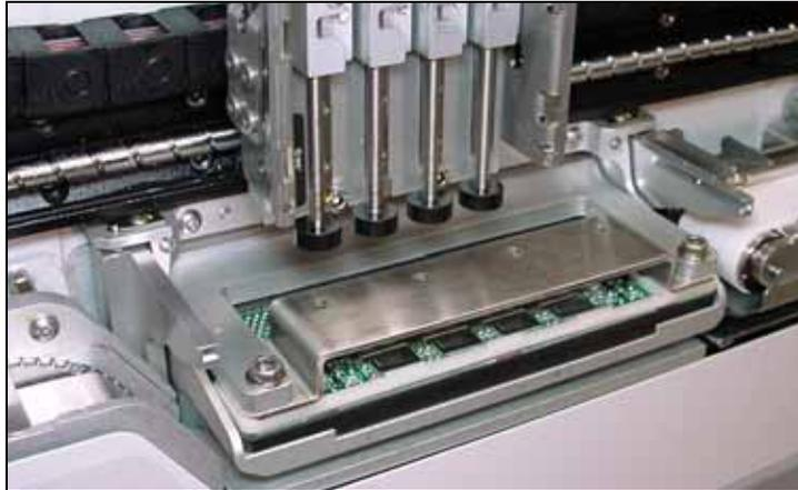
Figure U-43—The Programmer Module Alignment Tool Installed on the Programmer
