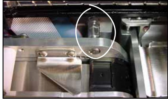
*Figure U-9—Some Tape-In Modules have an Adjustable Standoff for setting the Alignment with the Probes. The wrench flats and Locknut identify the Adjustment Stud from a non-adjustable Standoff.*
