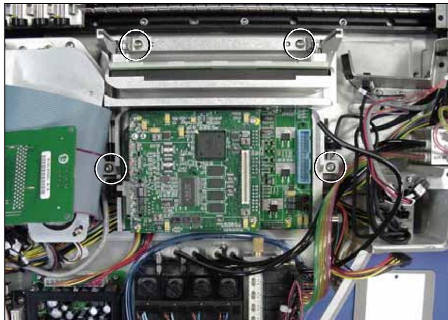
Figure U-42—Location of Programmer Screws
