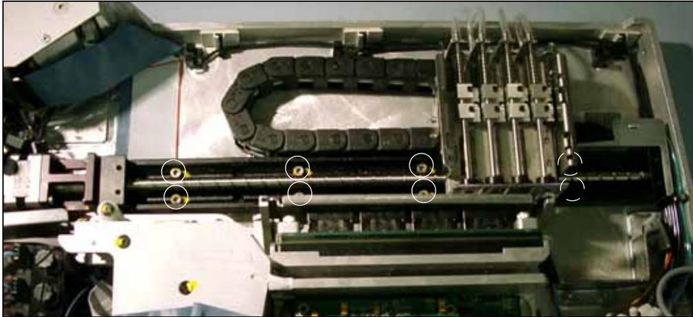
Figure U-53—Linear Stage Screw Locations. (Two are hidden by the head.)
