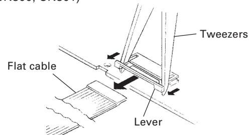
2. Gently rise up the connector lever in the direction of the arrow with a fine regular screwdriver or tweezers. (CN1, CN3, CN304)
