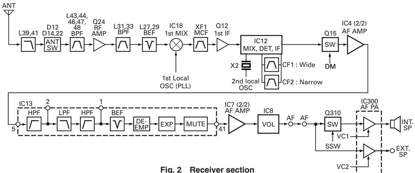
Fig. 2 Receiver section
