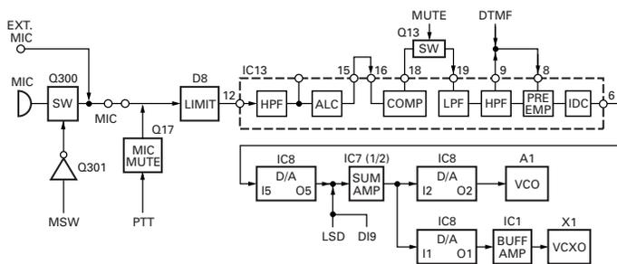
Fig. 7 Microphone amplifier
