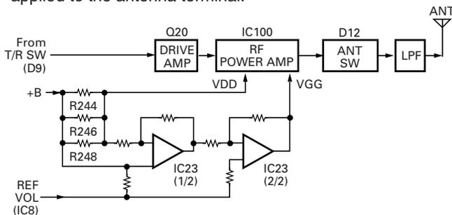
Fig. 8 Drive and final amplifier and APC circuit
