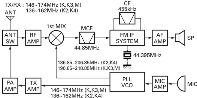
Fig. 1 Frequency configuration
