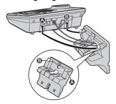
Adjust the adaptor to hold the base unit, then push it in the direction of the arrow until it clicks into place.
