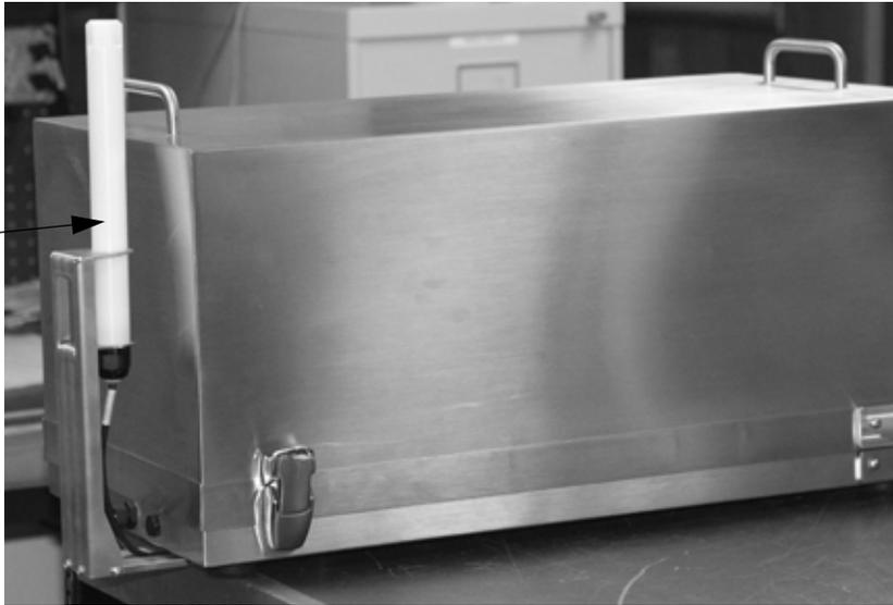
*Figure 5-41. Installed Wireless Antenna*
