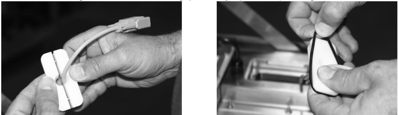
Figure 1-8. Assemble The Split Seal Plates Together
