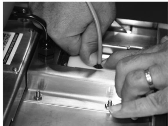
*Figure 1-11. Insert Split Grommet Onto the Split Seal Plates*
