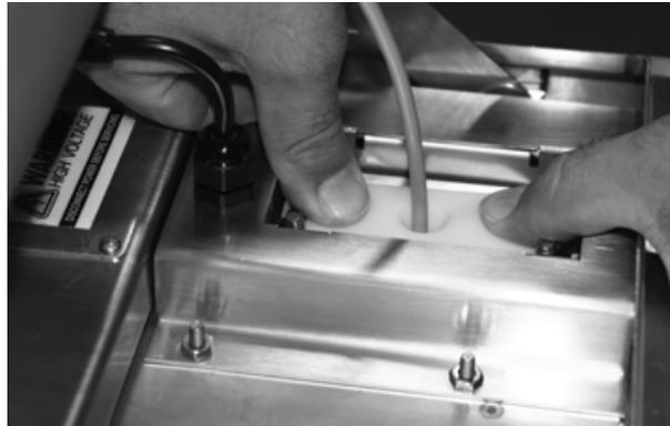
*Figure 1-10. Seat the Split Seal Assembly*
