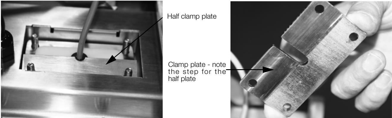
*Figure 1-12. Place Half Clamp Down on Assembly*
