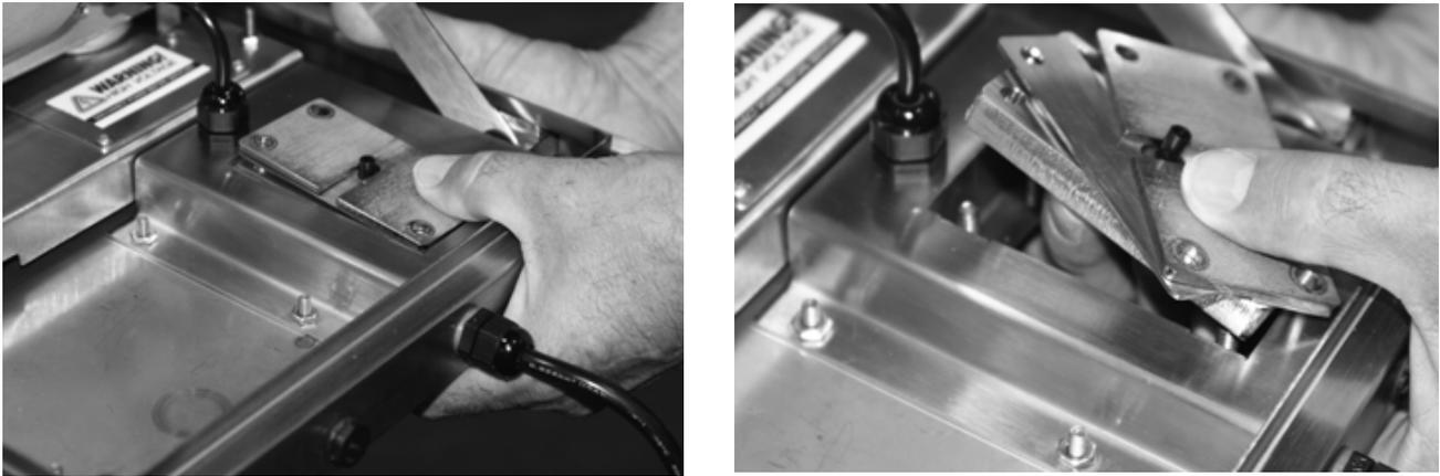
Figure 1-3. Remove the Component Parts of the Split Communications Cable Assembly
