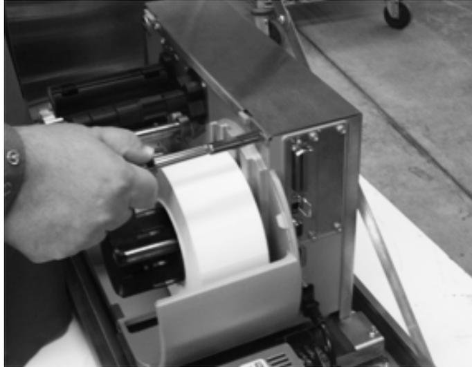
*Figure 3-3. Remove Screws from Enclosure*
