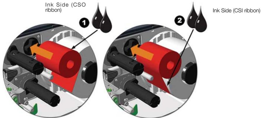
Figure 1-20. Wrap Ribbon Around Ribbon Spool
