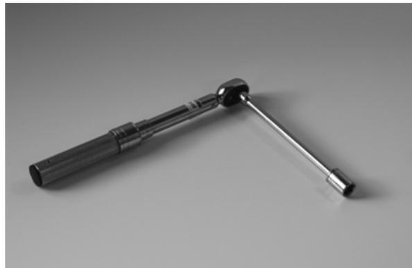
*Figure 1-14. 7/16" Socket and Torque Wrench Used to Tighten Assembly in Figure 1-13*
