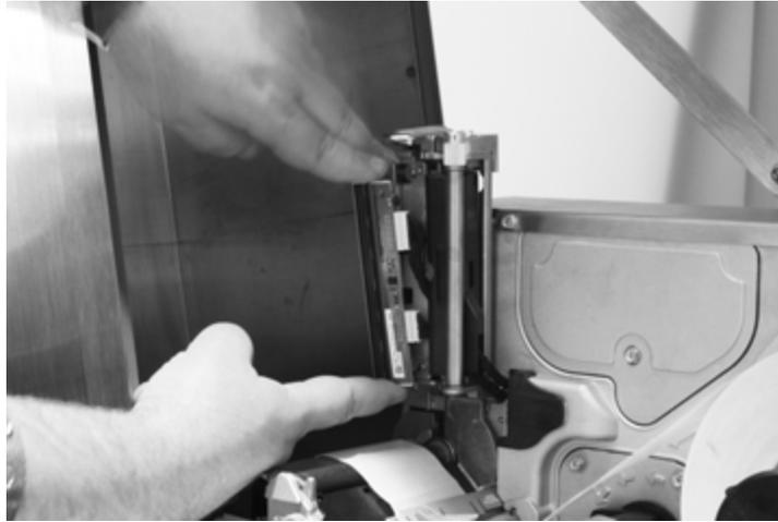
*Figure 3-2. Remove Old Printhead Assembly*
