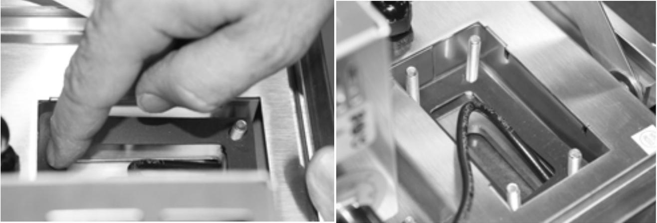
*Figure 5-31. Press Down Rubber Gasket Around Bolts*
