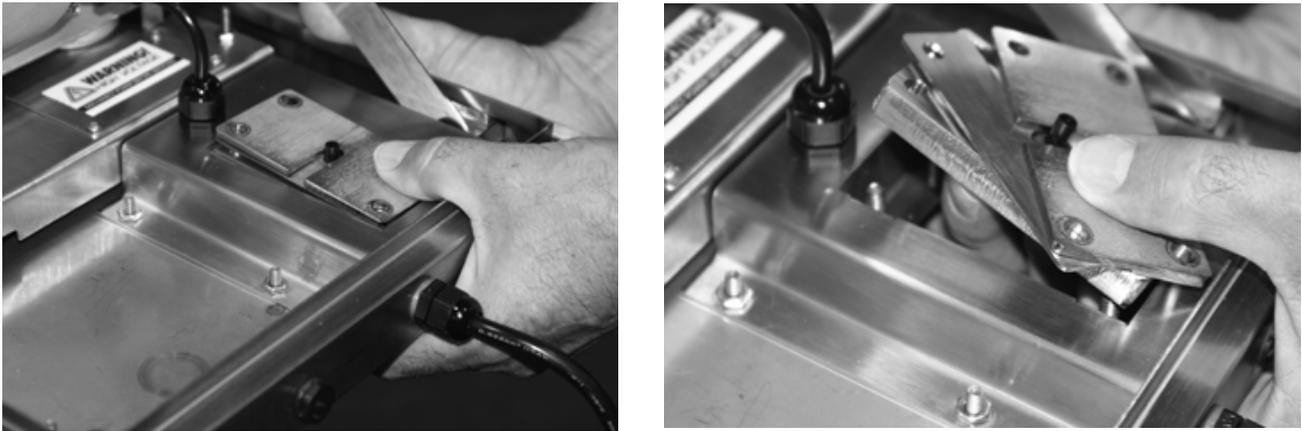
Figure 5-26. Remove the Component Parts of the Split Communications Cable Assembly
