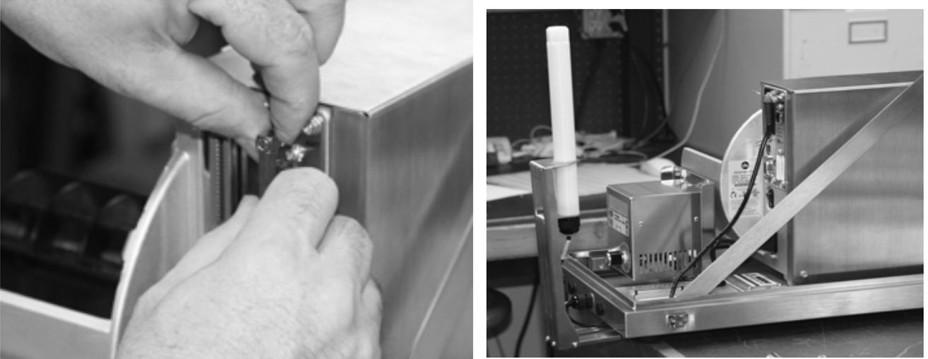
*Figure 5-34. Connect the Communications Cable to the Back of the Printer*
