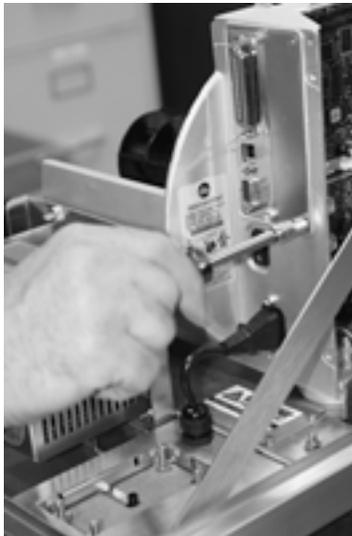
*Figure 5-21. Remove Screws from Cover Plate*
