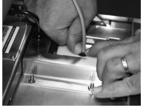
Make certain slack is present as shown in picture to allow sealing of cable to print case
