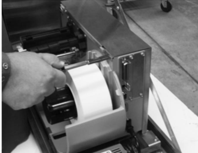
*Figure 5-20. Remove Screws from Enclosure*
