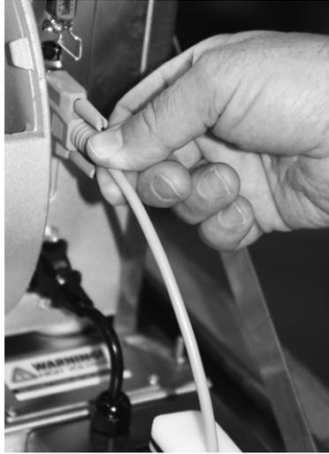
*Figure 1-9. Connect the Communications Cable to the Back of the Printer*
