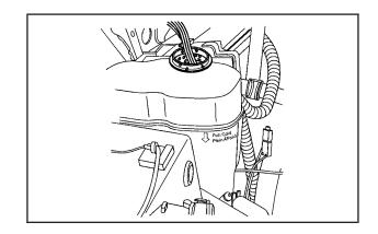
Fill the coolant surge tank with the proper mixture to the FULL COLD mark.
