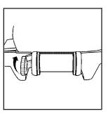
Unlatch the seat from the floor by lifting the lever located next to the carrying handle on the rear of the seat near the bottom.
