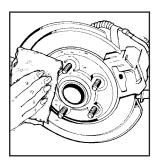
Remove any rust or dirt from the wheel bolts, mounting surfaces, and spare wheel. Put the wheel nuts back on with the rounded end of the nuts toward the wheel after mounting the spare tire.
