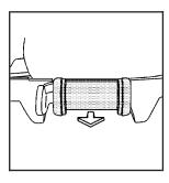
3. Unlatch the seat from the floor by pulling the carrying handle, located at the rear of the seat, rearward.
