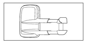
If the vehicle has towing mirrors, they can be adjusted for a clearer view of the objects behind you. Manually pull out the mirror head to extend it for better visibility when towing a trailer.
