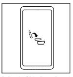
Press the automatic seat release button located on the panel behind the rear doors.
