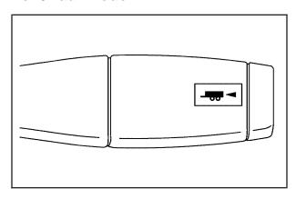
The vehicle has a Tow/Haul mode. The selector button is located on the end of the column shift lever. You can use this feature to assist when towing or hauling a heavy load or if there is a need to charge a battery installed in a trailer. See *Towing a Trailer on page 4-52* for more information.
