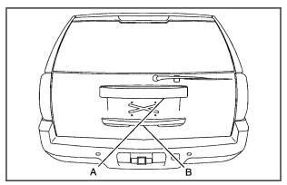
On vehicles with a liftglass, press the button on the underside of the license pocket applique (A) to open it. The liftglass can also be opened by pressing the liftglass release button on the RKE.
