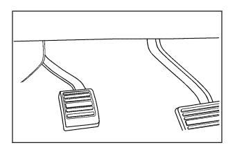
For vehicles without a release handle, set the parking brake by holding the regular brake pedal down, then pushing down the parking brake pedal.
