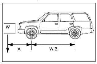
$(W \times (A + W.B.)) /W.B.=$  Weight the accessory is adding to the front axle.
