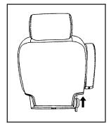
Lift the lever, located on the bottom rear of the second row seat on the inboard side, to release the seatback.
