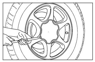
If your vehicle has a center cap that covers the wheel fasteners, place the chisel end of the wheel wrench in the slot on the wheel and gently pry the cap out.
