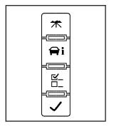
The buttons are the trip/fuel, vehicle information, customization, and set/reset buttons. The button functions are detailed in the following pages.
