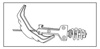
Tilt the tire toward the vehicle. Separate the tire/wheel retainer (G) from the guide pin. Pull the pin through the center of the wheel. Tilt the retainer down through the center wheel opening. Make sure the retainer is fully seated across the underside of the wheel.
