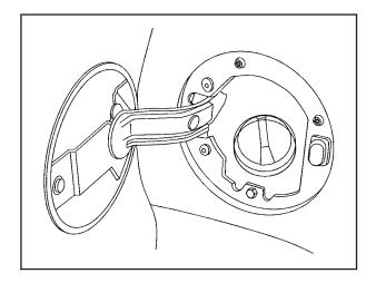
The tethered fuel cap is located behind a hinged fuel door on the driver side of the vehicle. If the vehicle has E85 fuel capability, the fuel cap will be yellow and state that E85 or gasoline can be used. See *Fuel E85* (85% Ethanol) on page 5-7.
