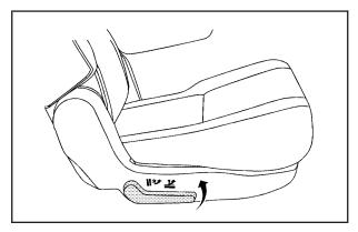
Lift the lever, located on the outboard side of the seat, to release the seatback.
