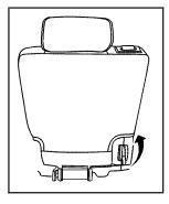
Lift the release lever, located on the bottom rear of the seatback on the outboard side of the seat, and the seatback will fold forward.
