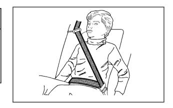
Buckle, position, and release the safety belt as described previously in this section. Make sure that the shoulder belt crosses the shoulder.
