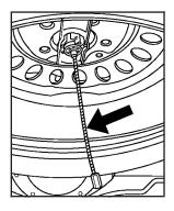
Check under the vehicle to see if the cable end is visible.
