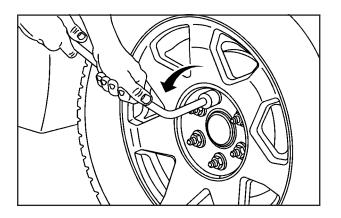
3. Use the wheel wrench to loosen all the wheel nuts. Turn the wheel wrench counterclockwise to loosen the wheel nuts. Do not remove the wheel nuts yet.
