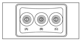
The A/V jacks, located on the rear of the floor console, allow audio or video signals to be connected from an auxiliary device such as a camcorder or a video game unit to the RSE system. Adapter connectors or cables (not included) might be required to connect the auxiliary device to the A/V jacks. Refer to the manufacturer's instructions for proper usage.
