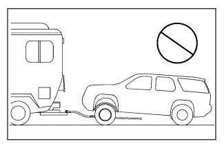
Notice: If a two-wheel-drive vehicle is towed with the rear wheels on the ground, the transmission could be damaged. The repairs would not be covered by the vehicle warranty. Never tow the vehicle with the rear wheels on the ground.
