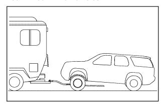
Use the following procedure to dolly tow a four-wheel-drive vehicle from the front:
