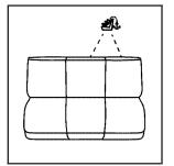
© (Top Tether Anchor): Seating positions with top tether anchors. There is one top tether anchor that can be used for either the third row center or driver side seating position but not both at the same time.
