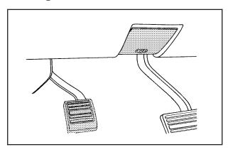
For vehicles with a release handle, set the parking brake by holding the regular brake pedal down, then pushing down the parking brake pedal.
