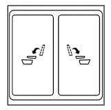
From the front seats, press one of the automatic seat release buttons located on the overhead console.
