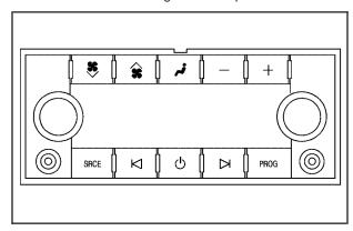
(Power): Press the U button to turn the RSA on or off.
