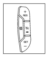
The cruise control buttons are located on left side of the steering wheel.
