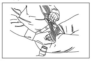
If the belt stops before it reaches the buckle, for lap-shoulder belts with cinching latch plates, tilt the latch plate and keep pulling the safety belt until it can be buckled.
