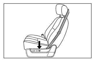
On seats with power lumbar, the controls used to operate this feature are located on the outboard side of the seats.
