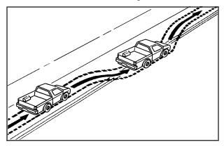
If the level of the shoulder is only slightly below the pavement, recovery should be fairly easy. Ease off the accelerator and then, if there is nothing in the way, steer so that the vehicle straddles the edge of the pavement. Turn the steering wheel 3 to 5 inches, 8 to 13 cm, (about one-eighth turn) until the right front tire contacts the pavement edge. Then turn the steering wheel to go straight down the roadway.
