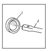
Insert the open end of the extension (J) through the hole in the rear bumper (I) (hoist shaft access hole).
