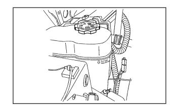
The coolant surge tank is located in the engine compartment on the passenger side of the vehicle. See *Engine Compartment Overview on page 5-14* for more information on location.
