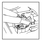
6. Connect the red positive (+) cable to the positive (+) terminal of the vehicle with the dead battery. Use a remote positive (+) terminal if the vehicle has one.
