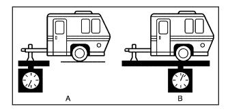
The trailer tongue weight (A) should be 10 percent to 15 percent of the total loaded trailer weight (B), up to a maximum of 600 lbs (272 kg) with a weight carrying hitch or up to a maximum of 1,000 lbs (453 kg) with a weight distributing hitch. For more information, see Weight-Distributing Hitches and Weight Carrying Hitches later in this section.
