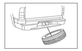
7. Tilt the tire toward the vehicle with some slack in the cable to access the tire/wheel retainer. Separate the retainer from the guide pin by sliding the retainer up the pin while pressing down on the latch.
