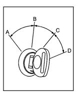
The ignition switch has four different positions.
