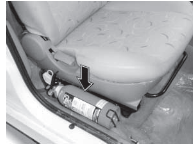
Fire extinguisher near Driver's Seat
