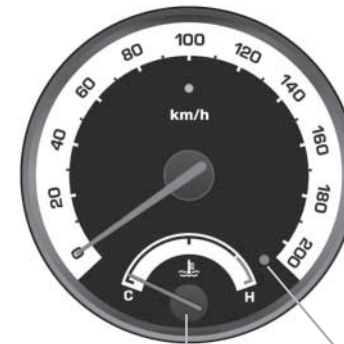
Temperature Gauge High Temperature Warning
