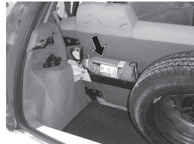
Fire extinguisher behind Rear Seat
