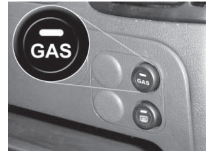
GAS Selector Switch
