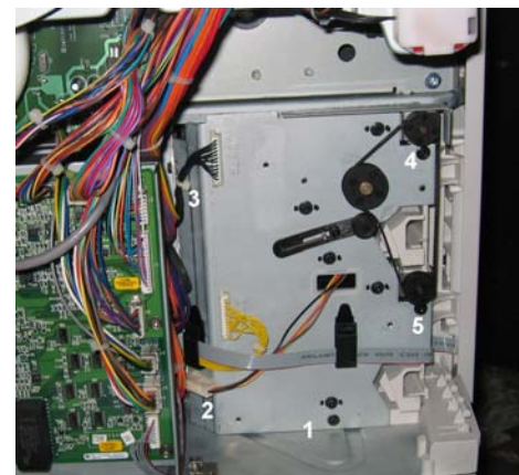
Photo 6 – Five Screws removes the Tray 1 & 2 Feed Module
