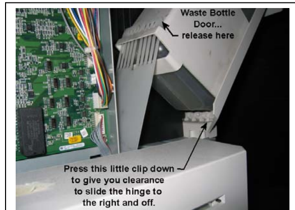
Photo 4 – Waste Toner Door Removal.
