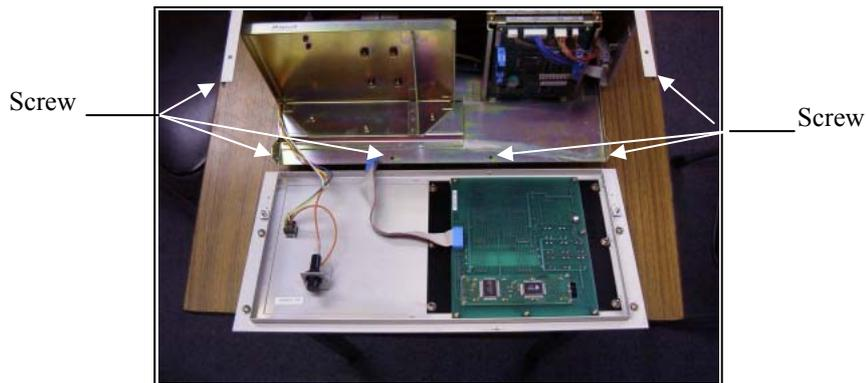
**Photo 4-6 Removal of display printed circuit board.**
