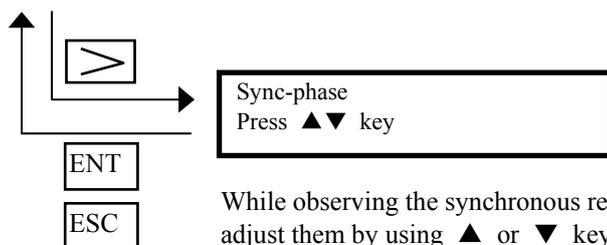
While observing the synchronous rectification waveforms with an oscilloscope, adjust them by using ▲ or ▼ key. Establish waveforms with the ENT key. If you want to stop halfway, press the ESC key.
