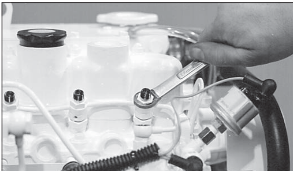
Figure 16: Remove return line nuts.
