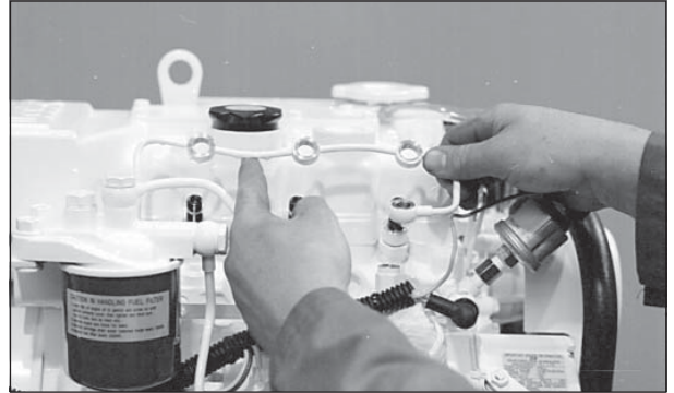
Figure 17: Remove return line.
