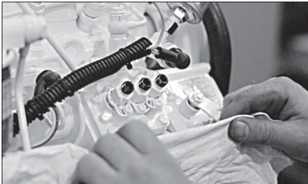
Figure 15: Cover lines, inlets and injection pump outlets.
