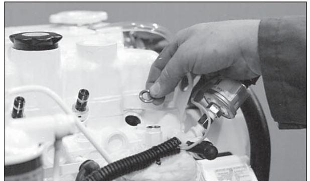
Figure 19: Remove and replace copper sealing washer.
