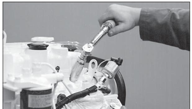
Figure 20: Reinstall injector. Torque to proper tightness.
