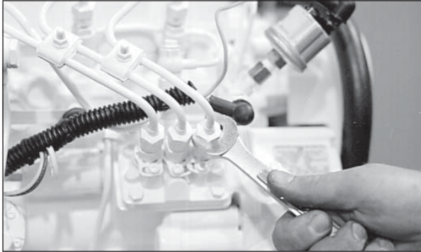
Figure 13: Remove delivery line flare nuts.
