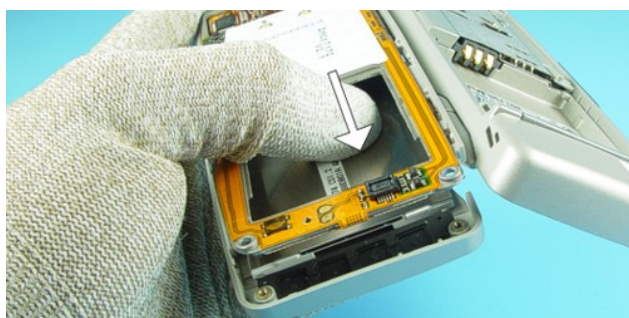
21.) Press out the C-Cover Assy carefully.
