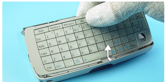
28.) Now, the Qwerty Keypad can be removed.
