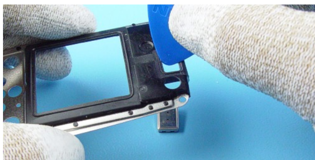
13.) Push out the Speaker with SRT-6.
