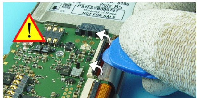
38.) Unlock the flex connector with SRT-6 carefully.
