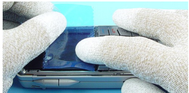
6.) Protect the LCD Module with a film.
