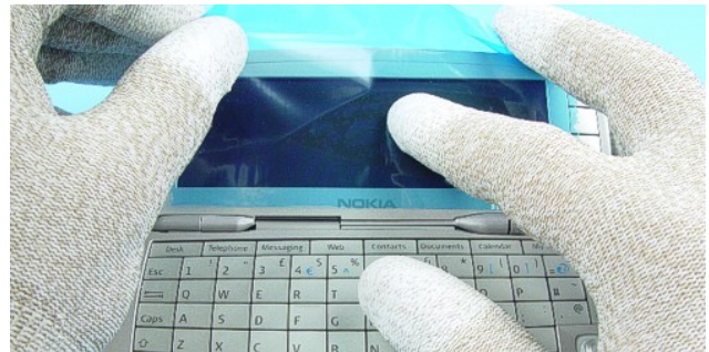
2.) Fit protective film to the LCD Module.
