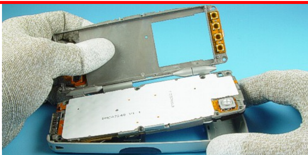
30.) Remove the Chassis Assy . Always start from the antenna side.
