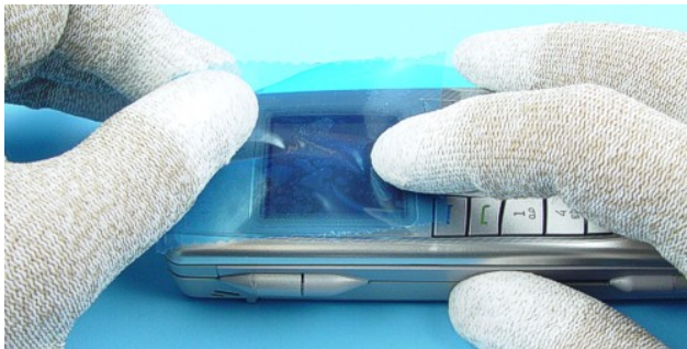
1.) Protect the window with a film.
