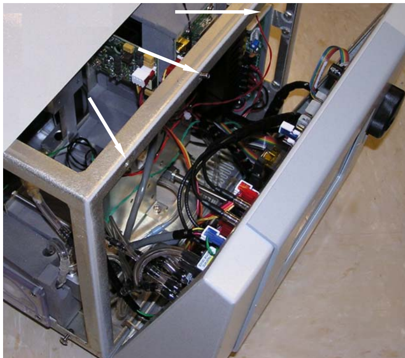
Figure 8-6 Front Panel Screw Removal
