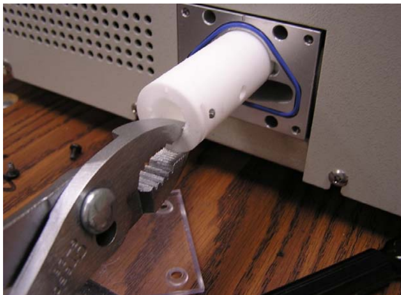
Figure 8-10 Pulling the Saturator Wick Out Using Pliers with Minimal Force
