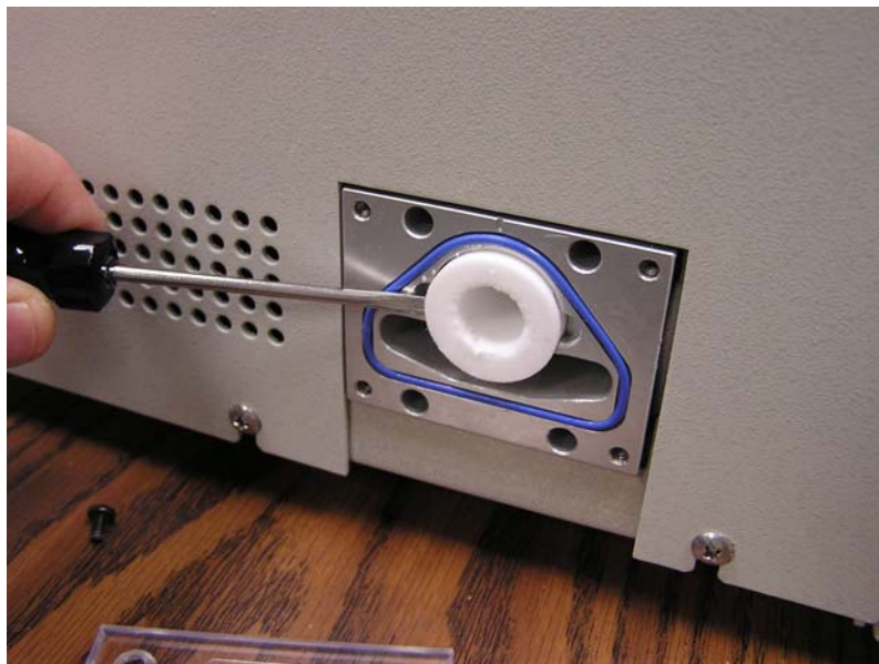
Figure 8-9 Prying the Saturator Wick Out
