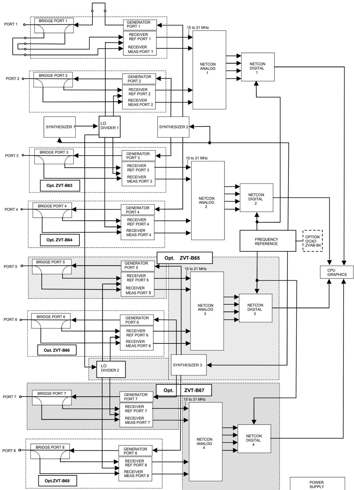
Fig. 3-3 Block diagram of the R&S ZVT8 8 ports with LO Divider 1300.2002
