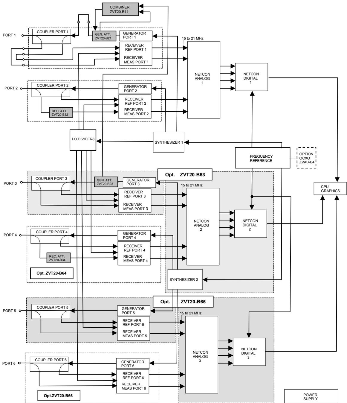
Fig. 3-5 Block diagram of R&S ZVT20 6 ports
