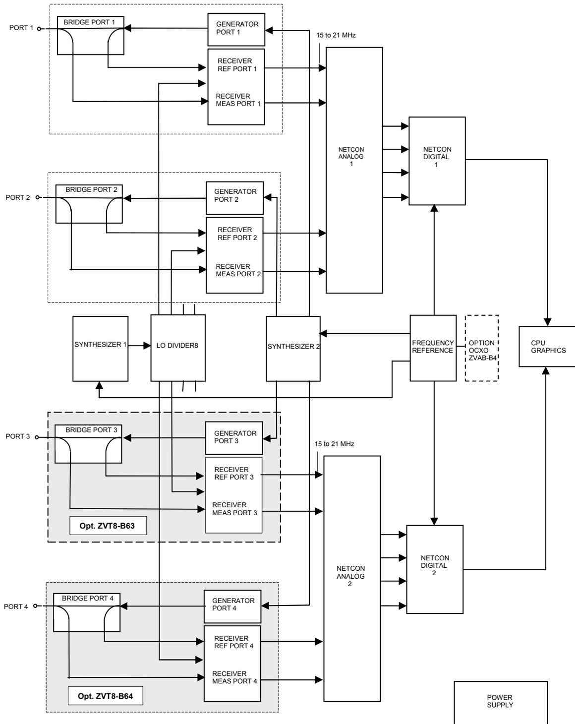
Fig. 3-2 Block diagram of R&S ZVT8 4 ports with LO Divider 8 1302.4060
