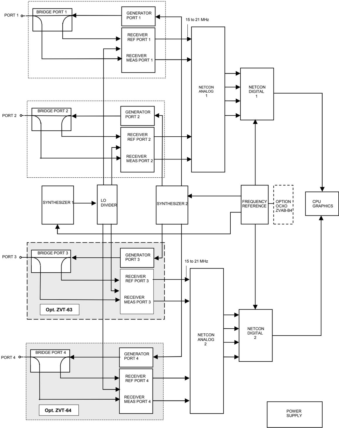
Fig. 3-1 Block diagram of R&S ZVT8 4 ports with LO Divider 1300.2002
