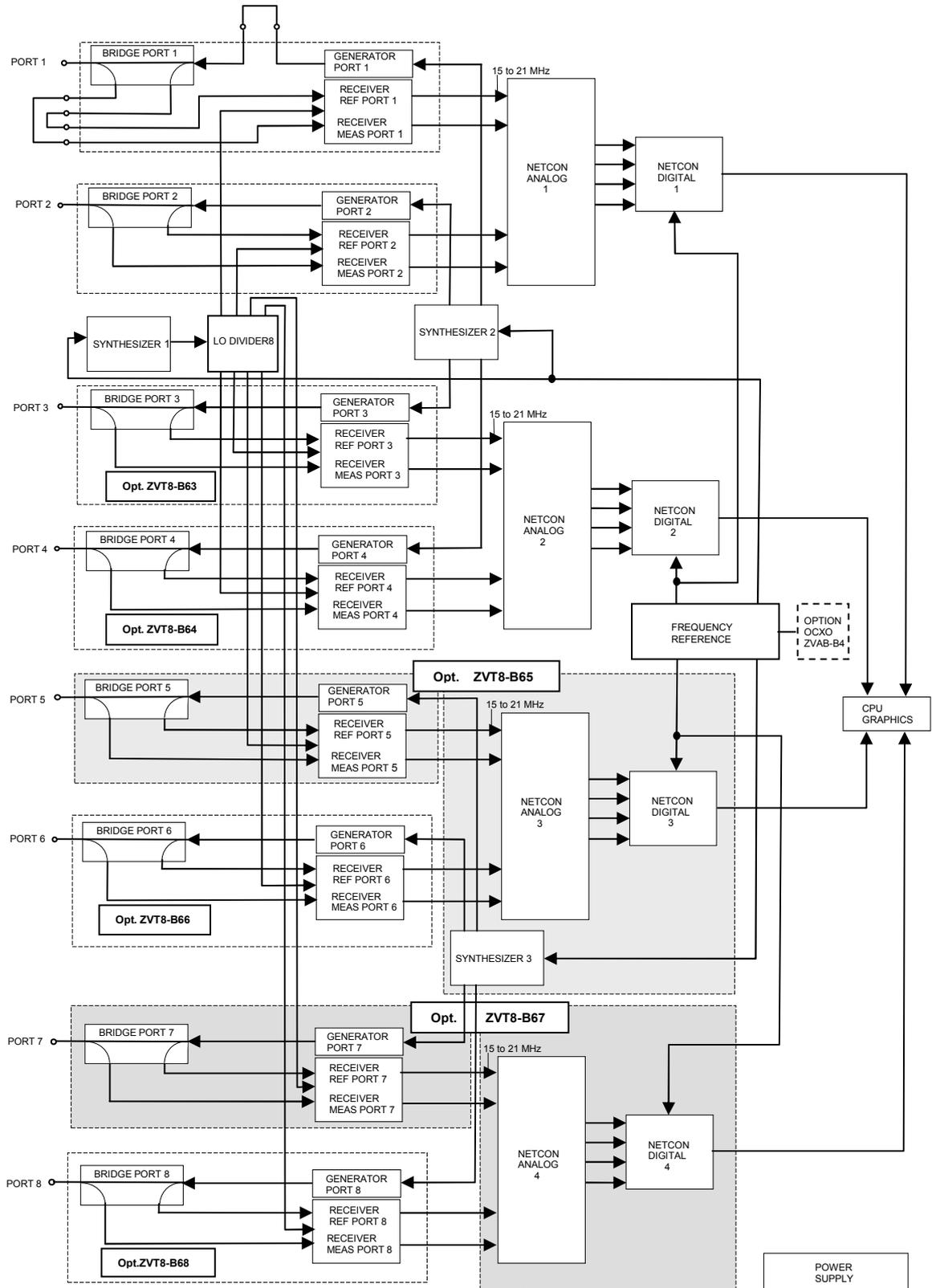
Fig. 3-4 Block diagram of R&S ZVT8 8 ports with LO Divider 8 1302.4060
