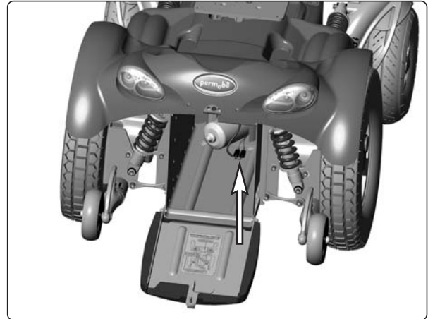
Seat elevator cabling.
