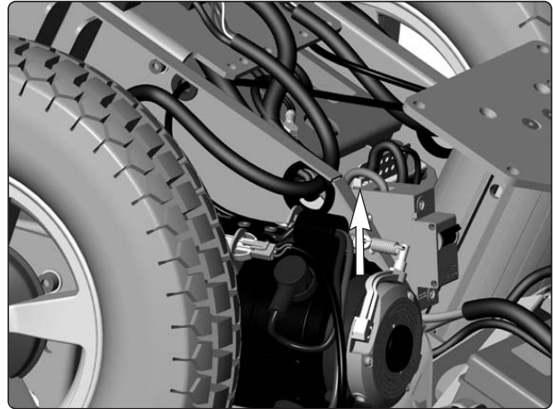
Circuit breaker bracket.
