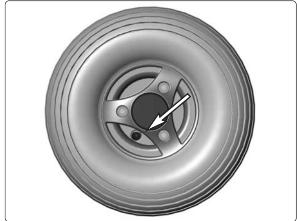
Filling Valve, front wheel.
