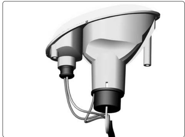
The light's insert and bulb holder. Fig. 78. The light's insert and bulb holder.
