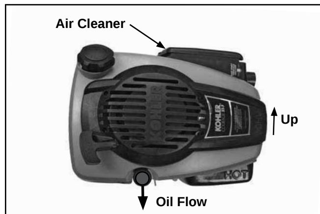
Figure 8-1. Draining Oil from Dipstick Tube.
