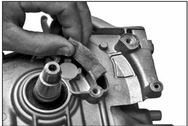
Figure 10-26. Installing Screen, Spring, and Disc.
