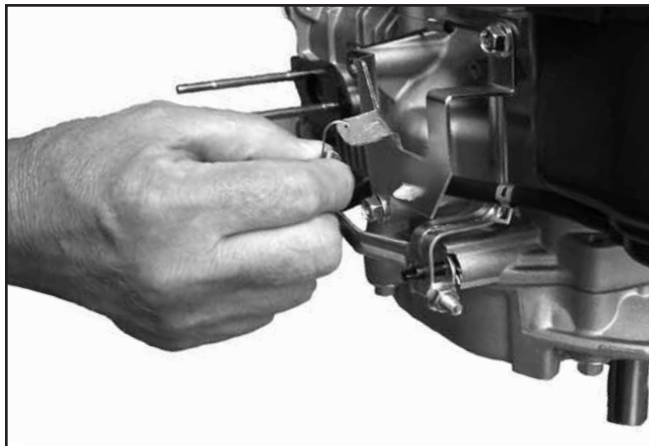
Figure 10-42. Installing Governor Spring.
