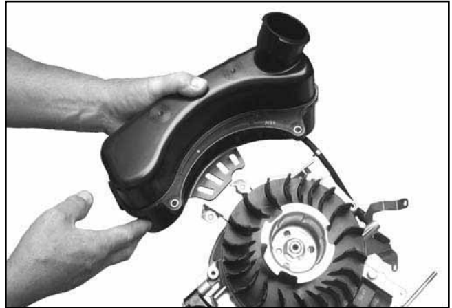
Figure 8-24. Removing Fuel Tank.
