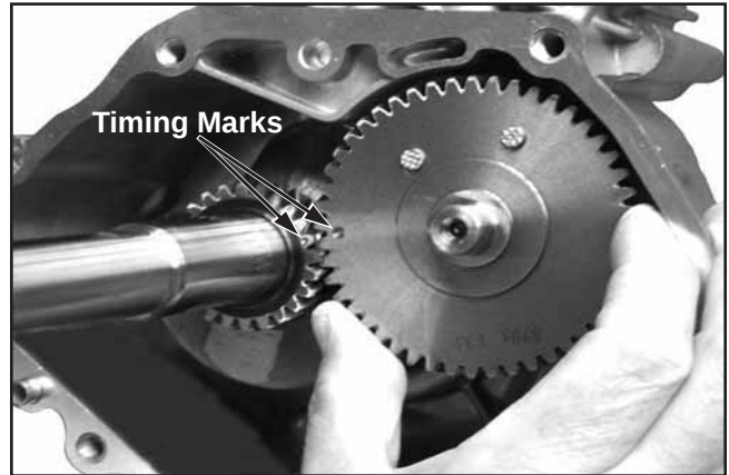
Figure 10-8. Aligning Timing Marks.
