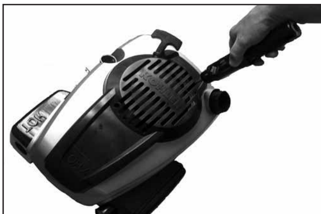
Figure 10-60. Installing Engine Cover Insert.
