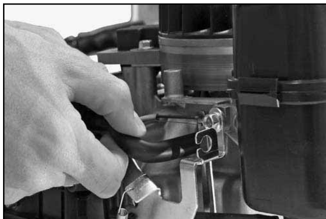
Figure 8-11. Detaching Breather Hose.
