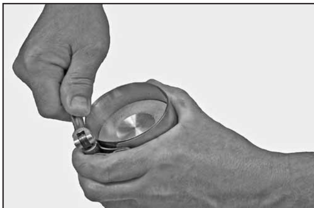
Figure 10-2. Compressing Piston Rings.
