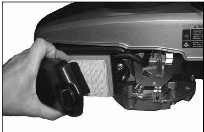
Figure 8-9. Removing Air Cleaner Cover.
