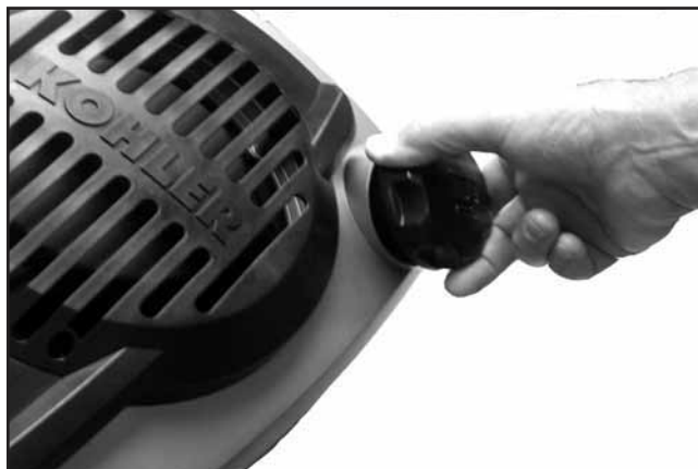
Figure 10-61. Installing Fuel Cap.
