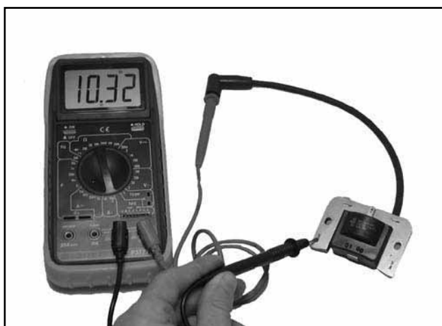
Figure 7-5. Testing CDI or IDI Ignition Modules.
