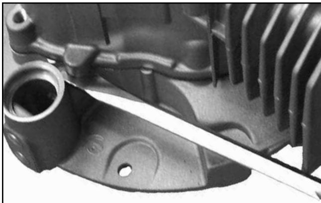
Figure 8-47. Separating Oil Pan from Crankcase.
