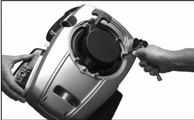
Figure 8-4. Removing Engine Cover.
