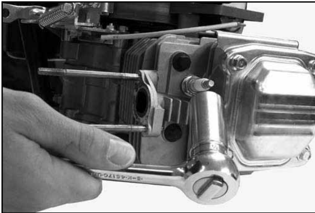
Figure 8-32. Removing Spark Plug.
