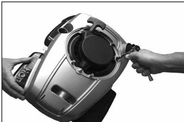
Figure 10-59. Installing Engine Cover.
