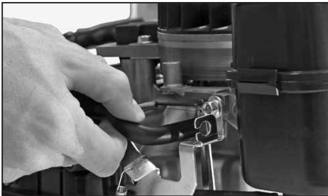
Figure 10-51. Attaching Breather Hose.
