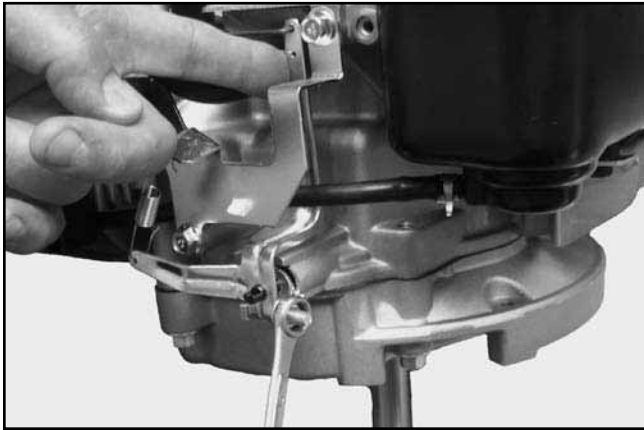
Figure 5-19. Loosen Governor Lever.
