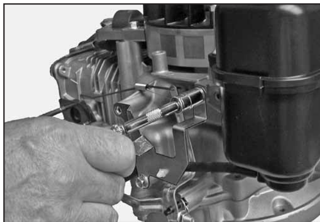
Figure 10-38. Installing Speed Bracket.
