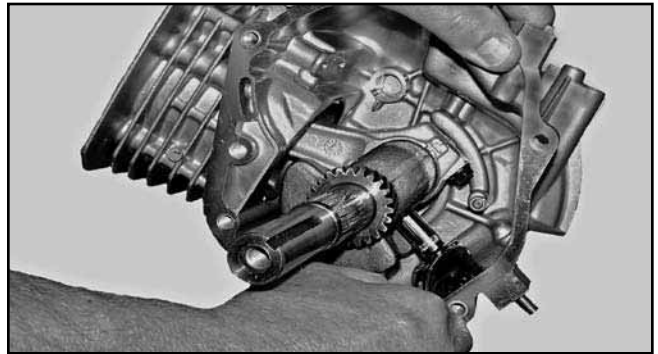
Figure 8-52. Removing Connecting Rod Cap.
