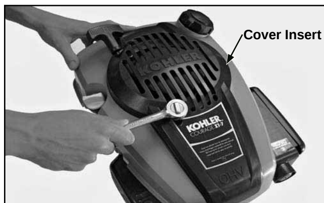
Figure 8-3. Removing Engine Cover Insert
