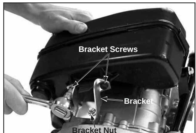
Figure 10-33. Attaching Fuel Tank Bracket.
