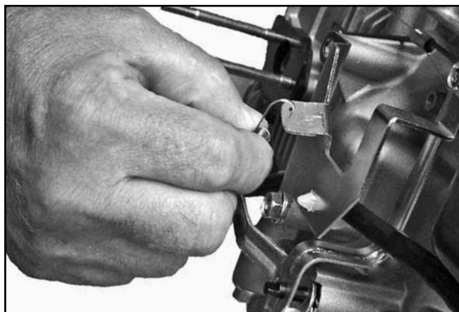
Figure 8-20. Removing Governor Spring.
