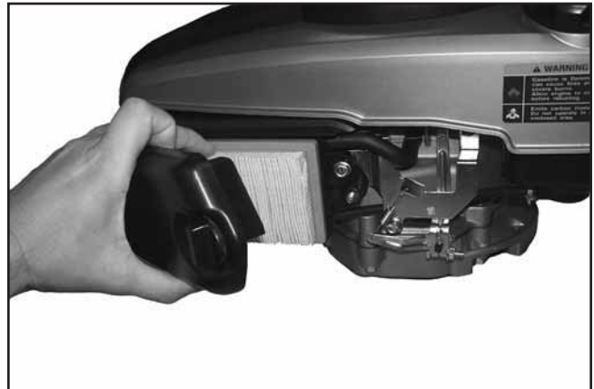
Figure 10-52. Installing Air Cleaner.
