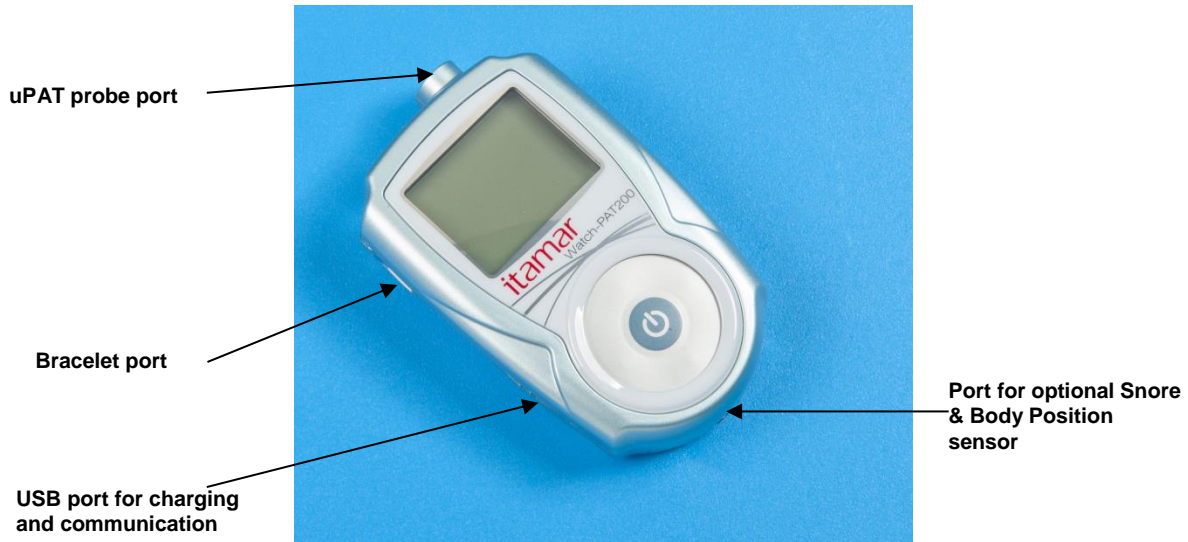
Figure 4 – Service Ports and Peripherals
