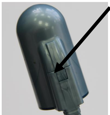
Figure 7 – Disconnecting the Probe
