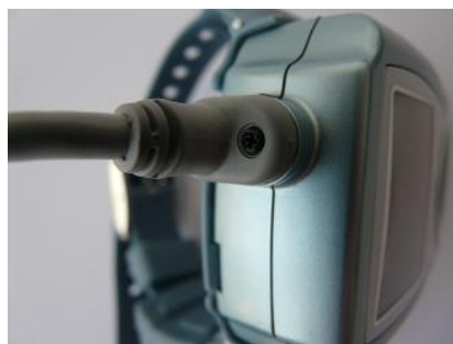
Figure 17 – uPAT Probe Cable with Screw
