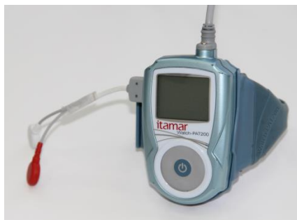
Figure 12 – WatchPAT™ Device with Cable for Bracelet
