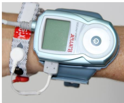
Figure 13 – WatchPAT™ Device with Bracelet
