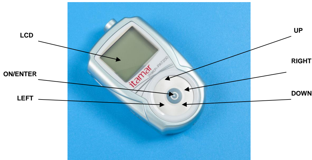
Figure 3 – The Buttons and Display
