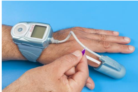
Figure 24 – Removing TOP Tab
