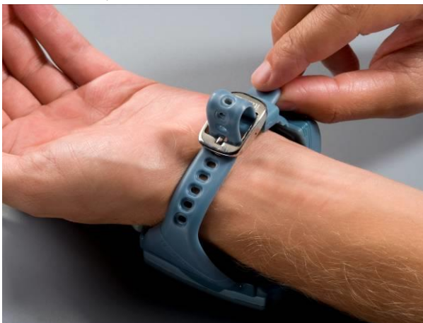
Figure 21 – Putting On The Wrist Strap
