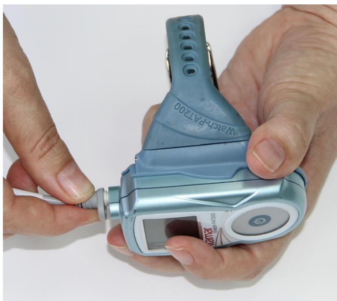
Figure 18 – Replacing the uPAT Probe
