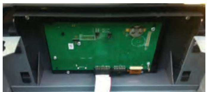
3. Remove bottom screws of the display panel.
