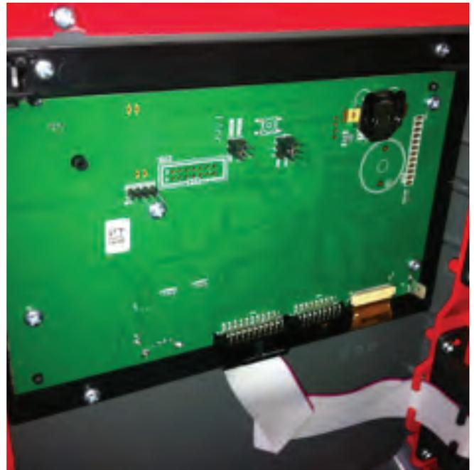
**CAUTION:** Use an anti-static wrist strap when removing and replacing circuit board assemblies.
