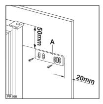
7. Place guide (A) on the inside part of the furniture door, upper and lower position as shown in the figure and mark the position of external holes. After having drilled holes, fix the guide with the screws supplied.
