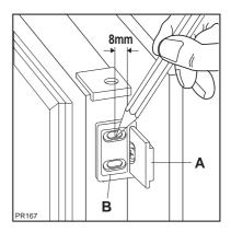
9. Open the appliance door and the furniture door at 90°. Insert the small square (B) into guide (A). Put together the appliance door and the furniture door and mark the holes as indicated in the figure. Remove the squares and drill holes with Ø 2 mm at 8 mm from the outer edge of the door. Place the small square on the guide again and fix it with the screws supplied.
