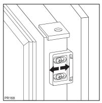
10. Should the lining up of the furniture door be necessary, use the clearance of slots. At the end of operations, it is necessary to check if the door of the furniture closes properly.
