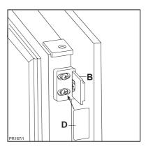
11. Fix cover (D) on guide (B) until it clips into place.
