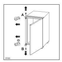
The appliance's door has been locked in position for transport by means of pins on both sides. According to the door opening direction, remove relevant pins at the top and at the bottom.
