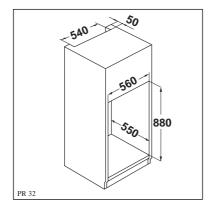
**1.** It is necessary that the cabinet has a ventilation recess with the following dimensions:
