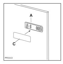
8. Fix cover (C) on guide (A) until it clips into place.
