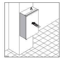
**2.** Push the appliance into the housing until stop strip (A) touches the kitchen unit.
