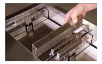
3. Lift the dispensing mechanism out of the dispenser by grasping the handles located on each side of the dispenser.
