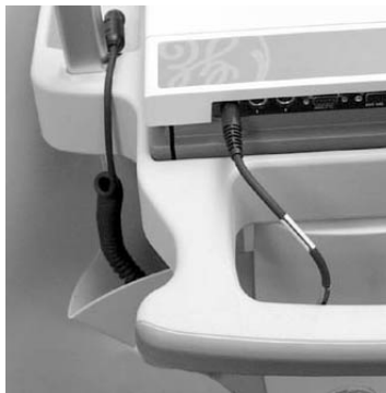
Correct amount of cable slack.
