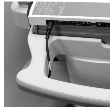
Not enough cable slack.
