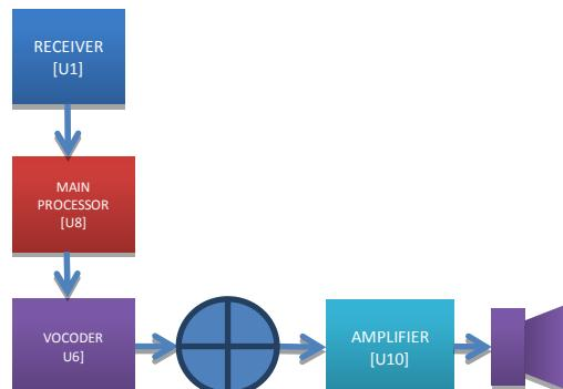
code, which de-encrypts the information, checks the integrity, corrects the wrong bits and extract the audio information form the received frame.
