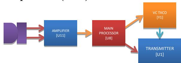
microphone (J4) are fed directly to the main processor (U8), which perform the signal filtering, the data codification, into especial firmware block. The result of the digitized information is processed by a FEC (Frame Error Correction) module, adding spare bits to ensure high robustness to the data, then it is encrypted and the user related information as user ID is added.
