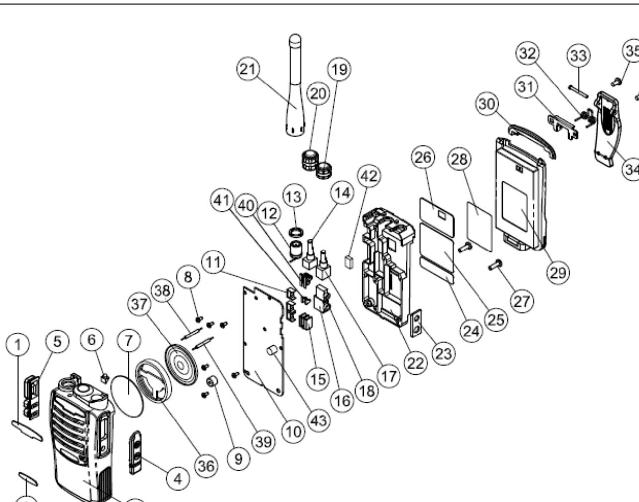
The diagram illustrates the exploded view of the SmarTrunk ST-1000 system. It shows the main chassis (22) with various internal and external components. External parts include the front housing (30), rear cover (30), antenna (21), ear jack cover (23), and belt clip base (31). Internal components shown in the exploded view include the battery pack (29), speaker (36), microphone (37), and various connectors and switches.
