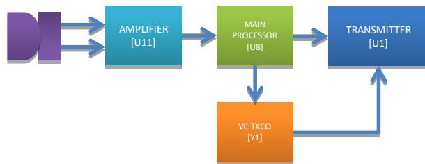
The AF signal from the internal microphone (MK1) or external microphone (J4) are processed as differential signal, then it is conditioned and transformed into common mode by the microphone pre-amplifier (U11).
