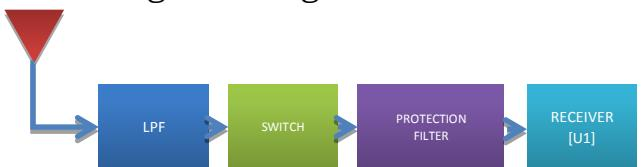
antenna are delivered to the Receiver Unit and pass through a Low-pass filter, antenna switching diode, and then fed to the receiver (U1) passing through a limiter BPF.
