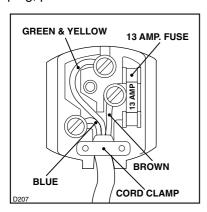
Connect the Green and Yellow (earth) wire to the terminal in the plug which is marked with the letter
