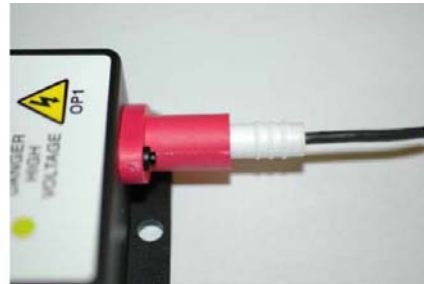
Cable Connected Loose (Incorrect)
