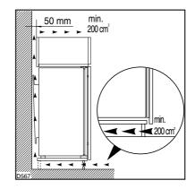
Furthermore, it is necessary that the cabinet has a ventilation recess with the following dimensions:
