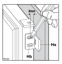
Remove the brackets and mark a distance of 8 mm from the outer edge of the door where the nail must be fitted (K).
