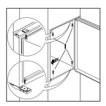
Apply the sealing strip pushing it between the refrigerator and the adjacent cabinet.
