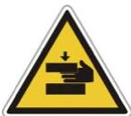
***To avoid the risk of crushing or amputation, only use this unit when its moving parts are fitted with correctly installed safety guards. Make sure all safety guards are correctly mounted after completing repair or maintenance work.***
