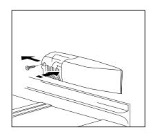
Unscrew the light cover and then pull it outward toward the middle of the cabinet. Unscrew the bulb and replace it with a new 25 watt bulb (available from your nearest Service Force Centre).
