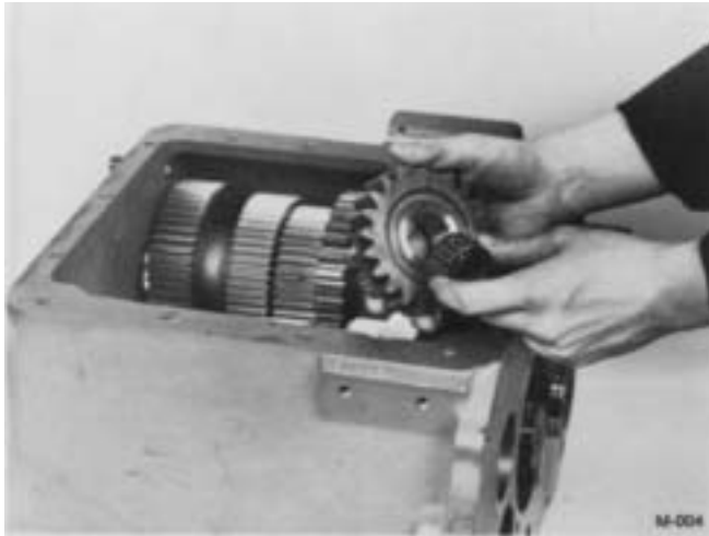
4. Remove the idler bearing from reverse idler gear.
