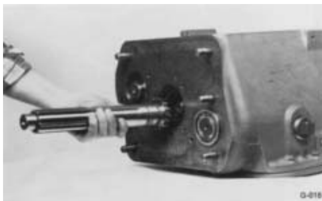
7. Pull shaft forward and from splines of drive gear.
