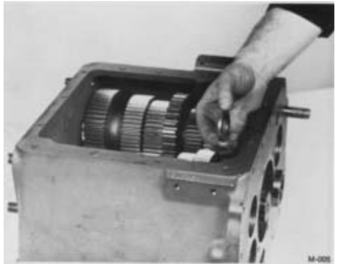
5. Remove the front idler washer from case
