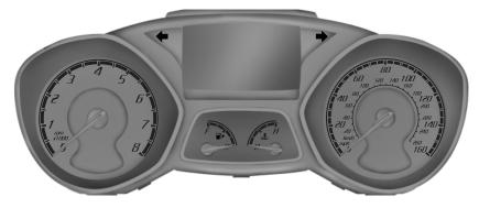
• ST high-speed instrument cluster and auxiliary cluster with oil temperature, oil pressure and boost gauges
