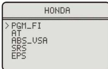
Systems that H685 supports here are classified 5 kinds, the operation ways of which respectively speaking are similar. Move [UP] or [DOWN] to move the cursors to choose what you need to enter to operate, and then press [Enter] to confirm. Here we choose **[AT]**. The screen will display the following.
