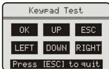
Press any key then the screen will flash due to corresponding to your cooperation. Double [Esc], you can withdraw from the testing.
