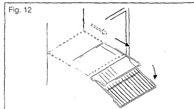
The shelves are designed to allow maximum air circulation and therefore when placing foods on the shelves make sure a small space is left between the packages.
