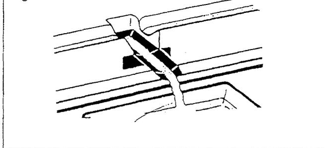
Scrape away as much frost as possible. Thawing of the remainder can be accelerated by placing bowls of hot water on the shelves inside the cabinet. As the solid frost loosens, prise it away with a wooden or plastic scraper. When defrosting is complete empty container. Wipe over the cabinet and the door with bicarbonate of soda and water and dry thoroughly as described under "Cleaning and Care".
