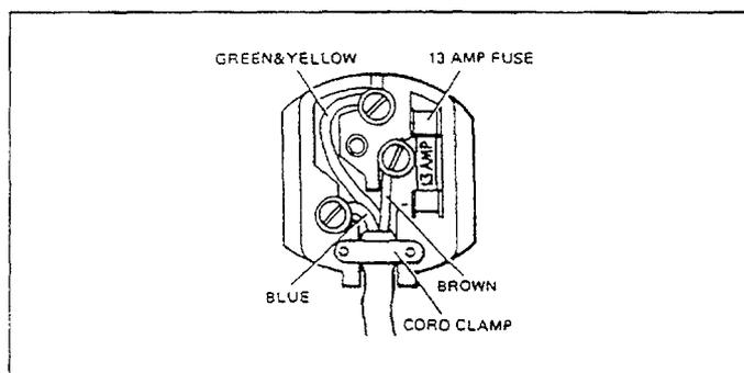
The appliance must be protected by a 13A ASTA approved (BS1362) fuse, if a 13A (BS1363) plug or a non rewirable plug is used, or if any other type of plug is used a 15A fuse either in the plug or adaptor or at the Distribution Board.
