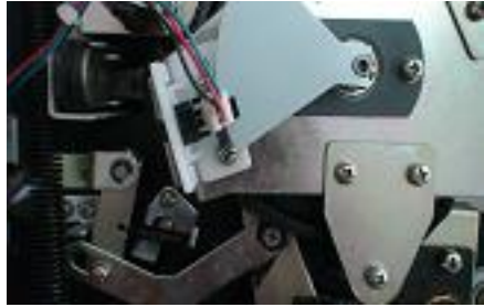
2 Clamper drive position sensor
