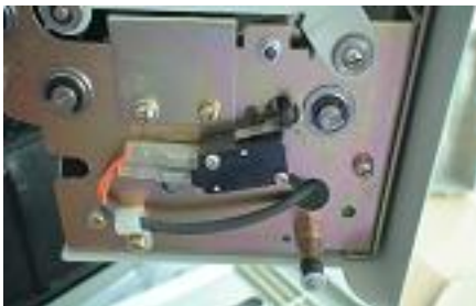
5 Disposal box full switch
