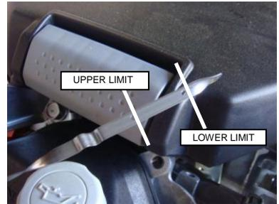
3. Remove the tank cap and check the fuel level.
