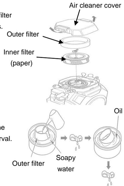
Inner filter (paper): Tap the filter element several times on a hard surface to remove dirt, or blow compressed air [not exceeding 207kPa(2.1kgf/cm<sup>2</sup>,30psi)] through the filter element from the air cleaner case side.
