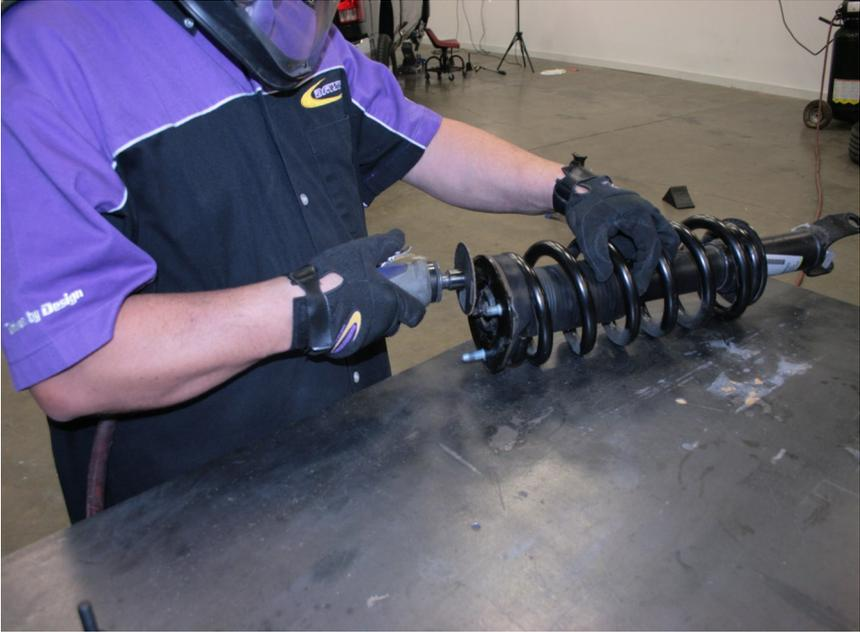
12. Install the stud extenders over the stock strut studs, and use the supplied Loctite
