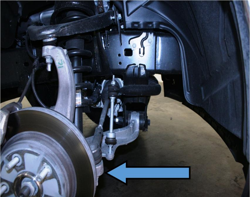
7. Remove the upper ball joint nut and separate the knuckle from the upper A-arm using the appropriate Puller tool
