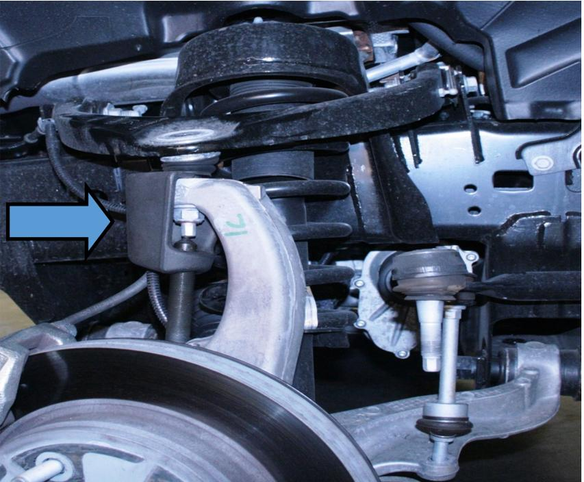
8. Remove the lower strut bolt and nut. Retain the factory lower bolt for reassembly. Note the direction of the bolt for reassembly
