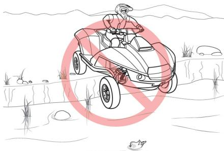
**⚠ WARNING!** Do not ride down a steep slope, off an undercut (for example, an eroded river bank,), a dock or other drop-off into the water. Ensure there are no obstacles or hazards at the entry point.
