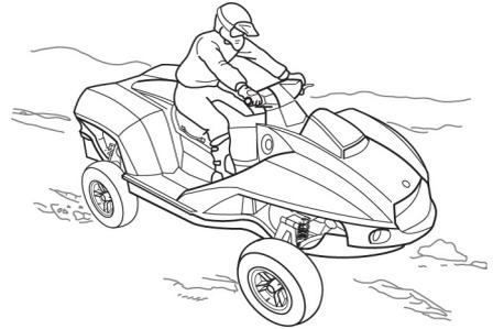
Do not descend a slope at high speed and avoid sudden braking or steering maneuvers as this could cause the amphibian to overturn.
