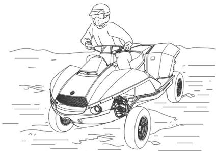
Terrain surface and speed are the major factors determining how the amphibian will react in a turn. Riding on loose, slippery or rough terrain (for example, snow, ice, mud, or gravel) makes it more likely for the amphibian to lose traction and skid or slide. This can result in a collision, or, if you unexpectedly regain traction, could result in the amphibian overturning. Stopping distances can also be longer.
