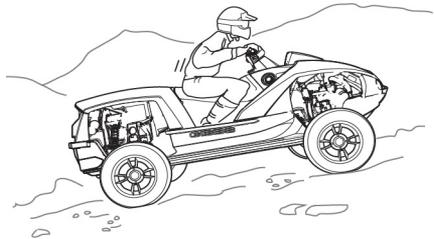
Before ascending a slope, slow down or stop to survey the terrain. When climbing a slope you must shift your weight toward the front wheels to help keep them on the ground. Move forward on the seat and lean forward.
