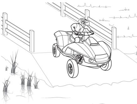
The most suitable and recommended access site is a hard slipway. If one is not available, then choose an entry point into the water that has a firm surface and gradual slope. Be sure that the waterway has sufficient depth for the draft of the hull and is free of underwater hazards and obstacles.
