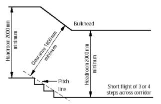
Additional headroom must be provided where short flights of three or four steps occur across a corridor. There is a tendency for some persons using such a flight to jump down all the steps at once. In these circumstances, the clearance should be at least 1800mm (see illustration). A bulkhead should be incorporated rather than a down-stand beam whenever a short flight occurs across a corridor.
