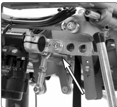
Fig. 10. Front actuator bracket for the backrest actuator on the Junior seat, positions A, B and C.
