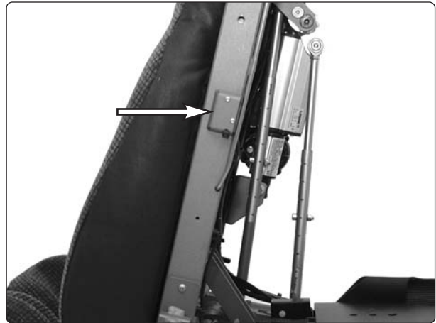
Fig. 67. The crush-protection sensor is mounted on the left side of the seat frame.
