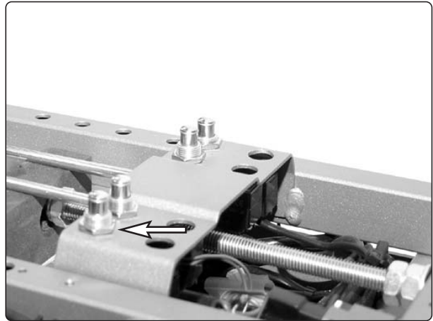
Fig. 58. The sensor is mounted with a nut.
