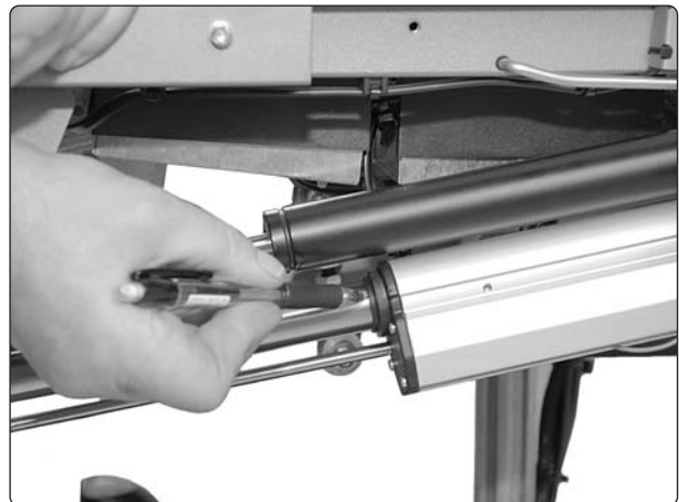
Fig. 80. Mark the piston of the stand function actuator.
