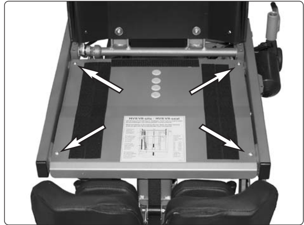
Fig. 91. The seat plates are mounted using four screws.
