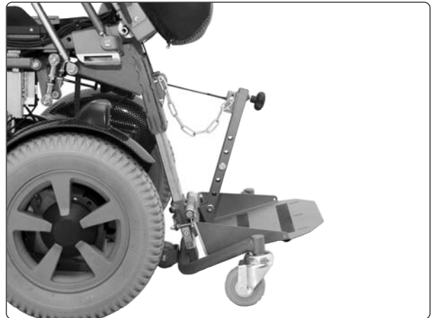
Fig. 41. Angle of the knee stops strap in the standing position.
