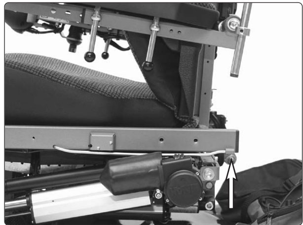
Fig. 2. The rear fastener of the crush-protection sensor is mounted using a screw underneath it.
