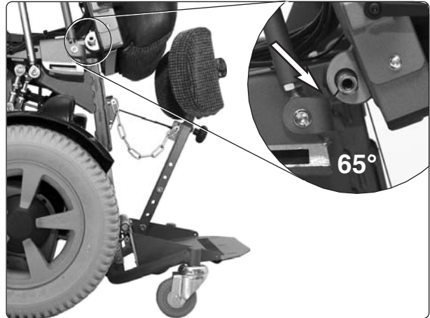
Fig. 36. The support wheel must be touching the floor when the seat is raised to an angle of 65°.
