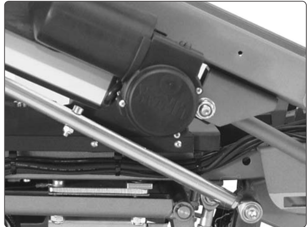
Fig. 86. The electrical connections are located behind a protective cover.
