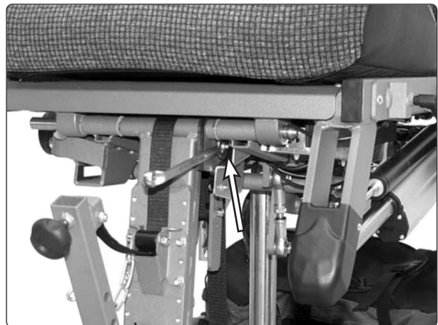
Fig. 31. The nut locks the angle of the cam disk.
