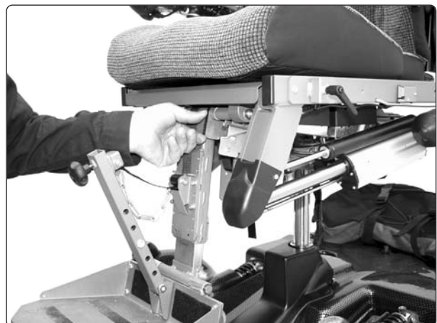
Fig. 32. Adjust the angle of the cam disk.
