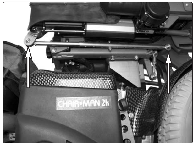
Fig. 84. The parallel strut is mounted with two screws, the parallel strut for the back/legs is shown in the picture.
