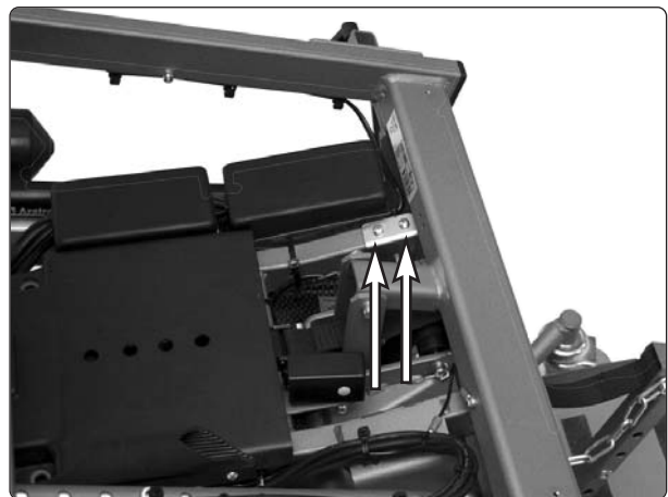
Fig. 63 The plate with the sensors is mounted with two screws.
