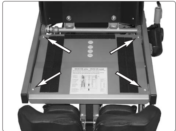
Fig. 13. The seat plates are mounted using four screws.
