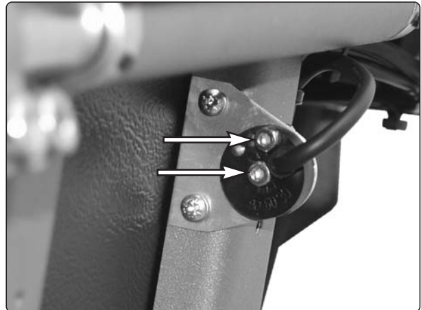
Fig. 72. The angle stop is mounted using two screws.
