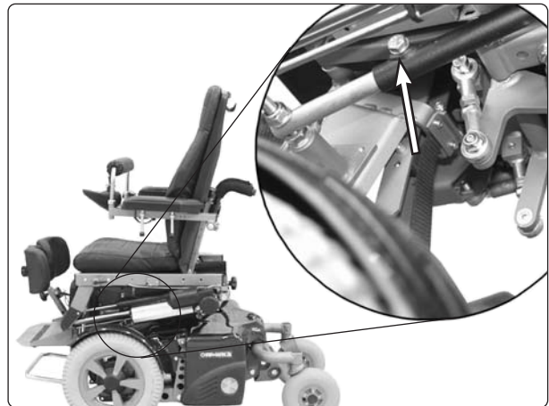
Fig. 27. Setting the slope of the leg rest.
