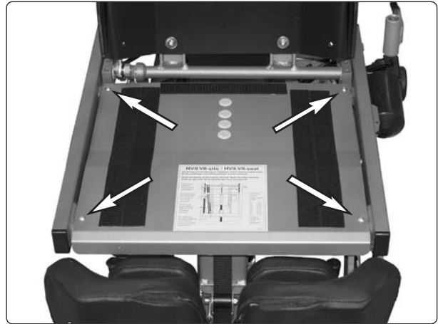
Fig. 51. The seat plates are mounted using four screws.
