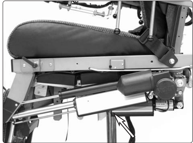
Fig. 54. The combi relay box is located underneath the seat function board's case.
