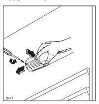
Unscrew the light cover and then pull it outward by pressing as shown in the figure. Unscrew the bulb and replace it with a new 15 watt bulb (available from Expert Appliance Care).
