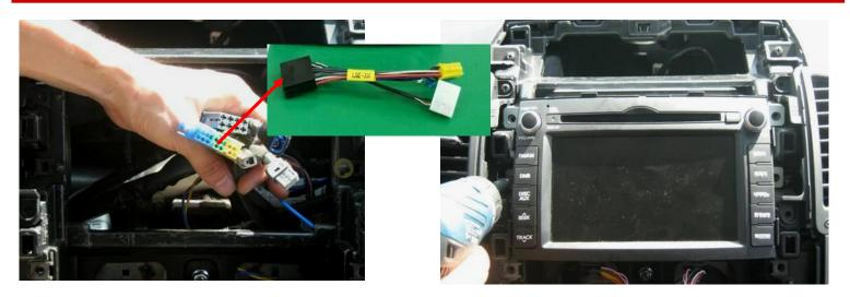
7.Connect the extension connector between original connector and AVN head unit for camera.
