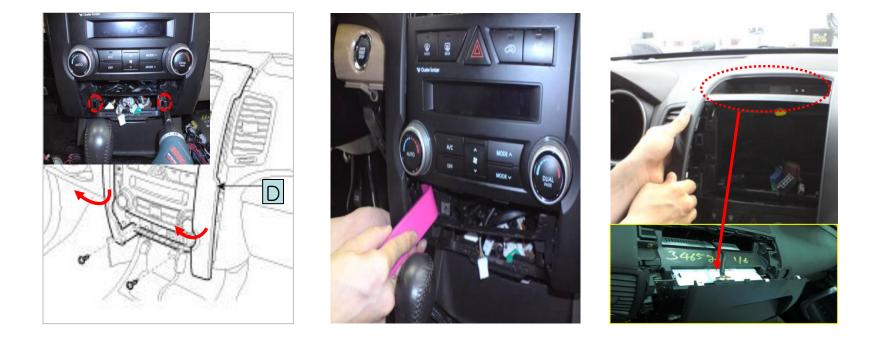
5. After removing two screws , carefully pry off the center facia panel "D" and disconnect the clock connector.
