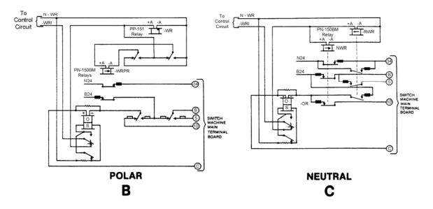
NOTE: EXTERNAL CONNECTIONS ARE SHOWN TO THE MAIN TERMINAL BOARD FOR A SWITCH HAVING THE RIGHT-HAND POINT NORMALLY CLOSED.
