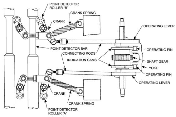
Figure 2–10 - Schematic Diagram of Point Detector - Parts in Reverse Position
