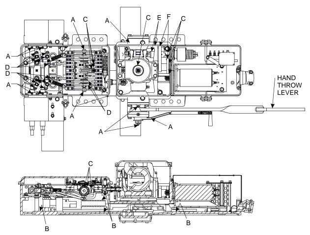
Figure 5-4 - Lubrication Diagram for M-23A, M-23B Switch Machine
