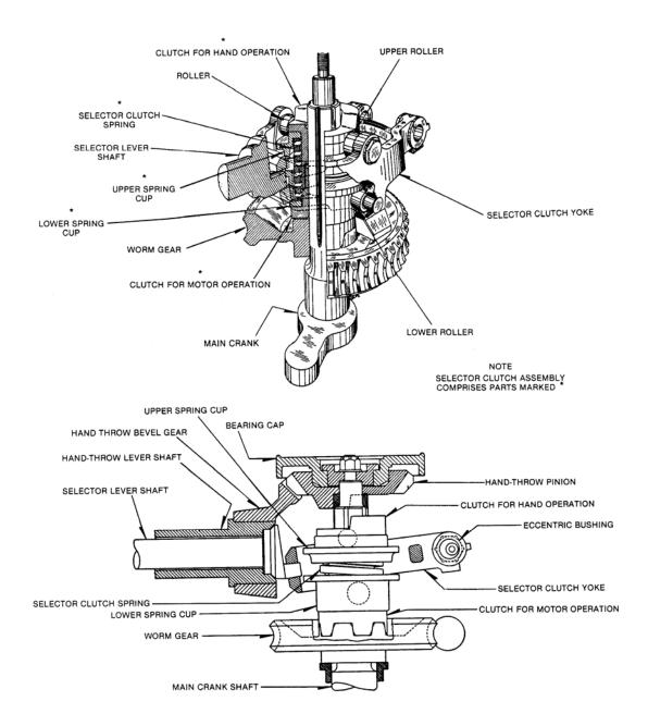
Figure 2-14 - Sectional Views of M-23A Dual-Control Mechanism
