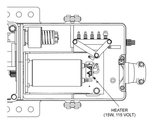
HEATER FOR MOTOR COMPARTMENT
