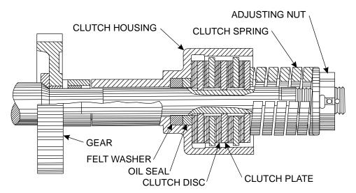
Figure 5-2 - Friction Clutch Assembly
