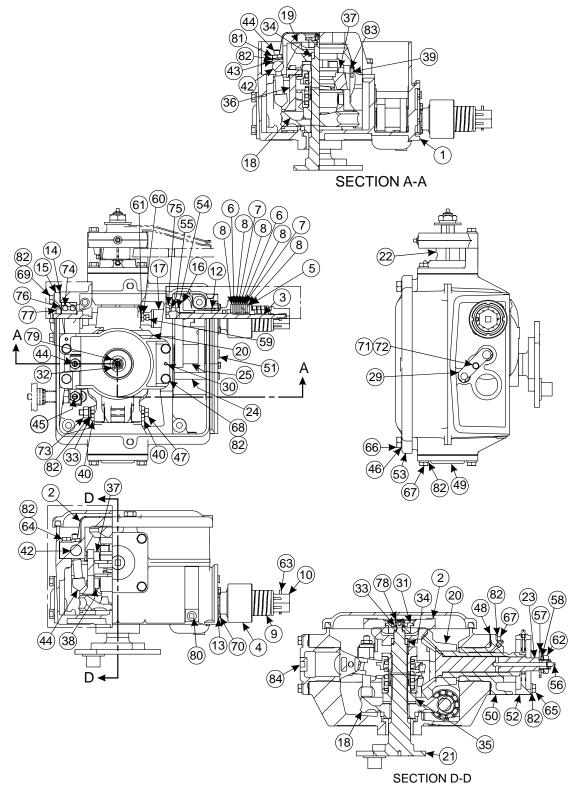
Figure 7-4 - M-23A/M-223B IPD Switch Machine Gearbox
