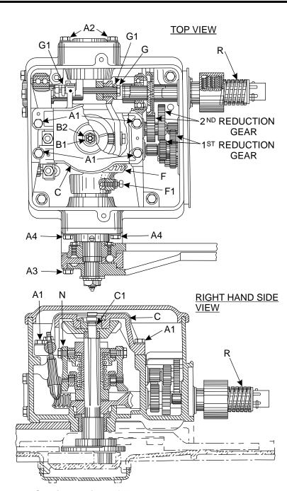
Figure 2-12 - Sectional View of M-23A Gearbox
