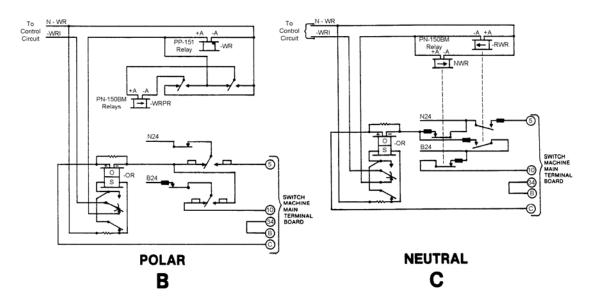
NOTE: EXTERNAL CONNECTIONS ARE SHOWN TO THE MAIN TERMINAL BOARD FOR A SWITCH HAVING THE RIGHT-HAND POINT NORMALLY CLOSED.
