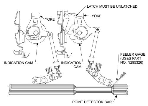
Figure 5-6 - Latch in Unlatched Position
