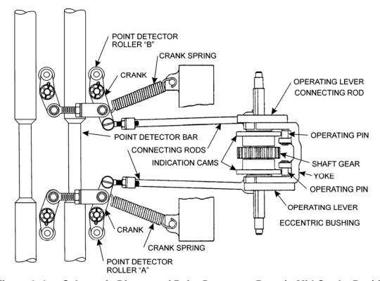
Figure 2-9 - Schematic Diagram of Point Detector - Parts in Mid-Stroke Position
