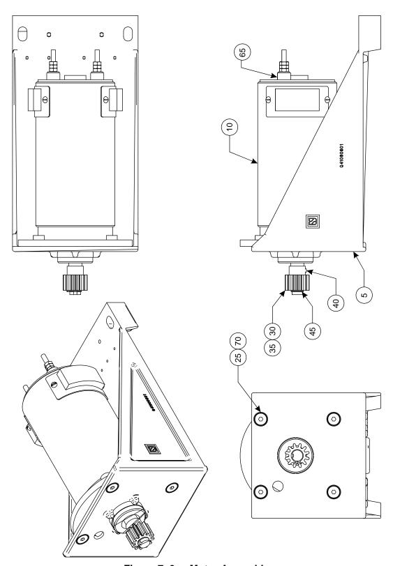
Figure 7-6 - Motor Assembly
