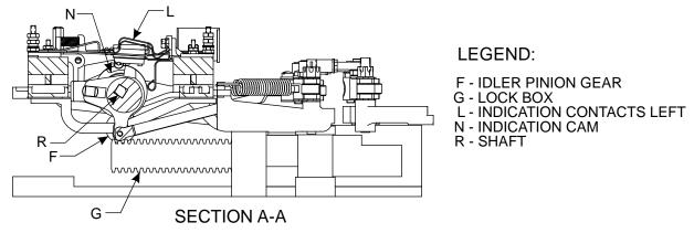
Figure 2–6 - Sectional View of Indication Circuit Controller
