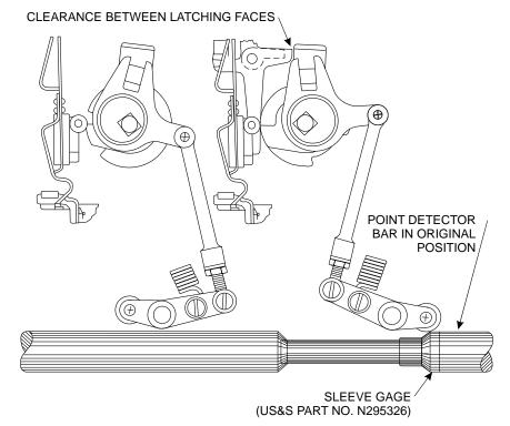
Figure 5-7 - Inserting the Sleeve Gage
