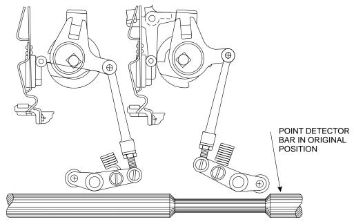
Figure 5-8 - Contacts in the Open Position
