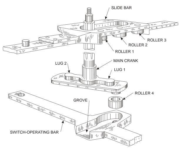
Figure 2-1 - M-23A and M-23B Switch Operating Mechanism
