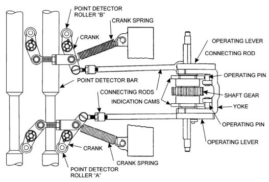
Figure 2–8 - Schematic Diagram of Point Detector – Parts in Normal Position
