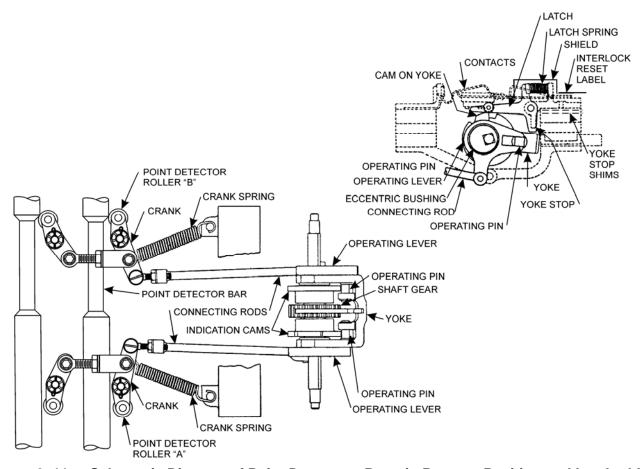
Figure 2-11 - Schematic Diagram of Point Detector - Parts in Reverse Position and Latched-Up
