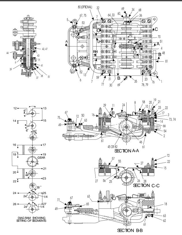
Figure 7–5 - M-3, M-23A, and M-23B IPD Switch Machine Circuit Controller Parts Location
