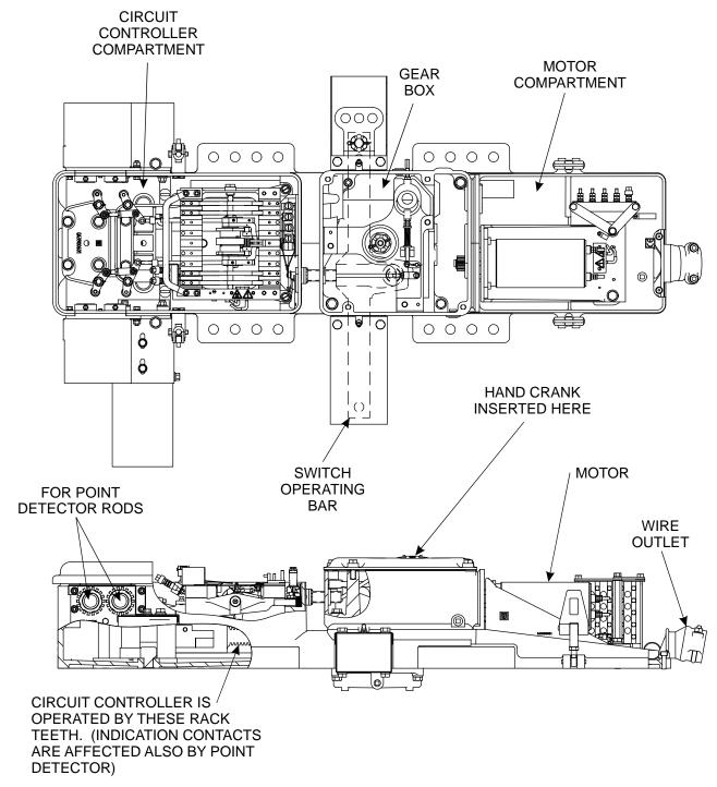
Figure 1-1 - Outline Diagram of the M-3 Switch Machine
