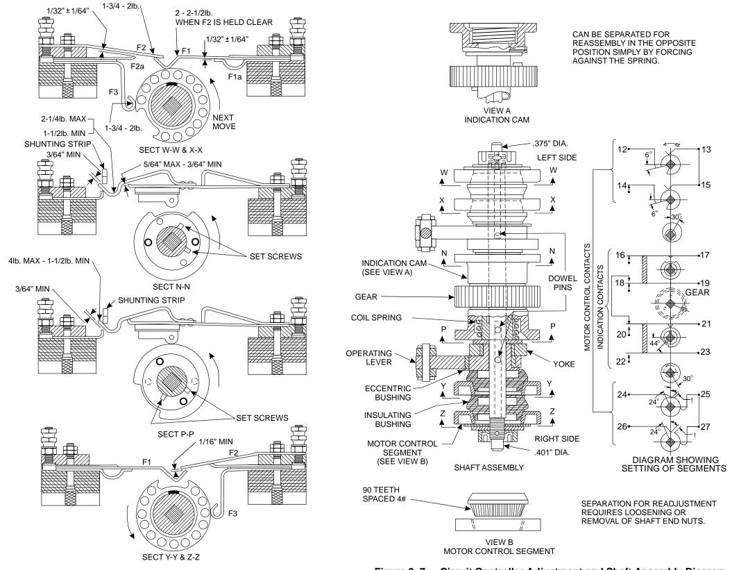
Figure 2-7 - Circuit Controller Adjustment and Shaft Assembly Diagram
