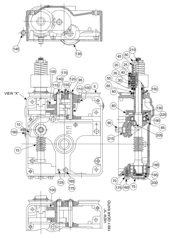
Figure 7-3 - M-3 IPD Switch Machine Gearbox
