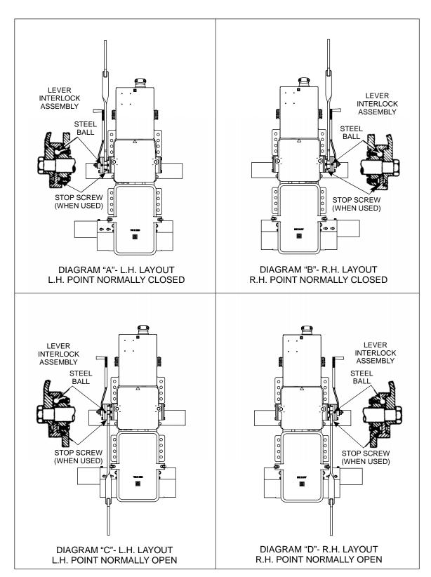
Figure 3-9 - Standard Lever Interlock Assemblies for Style M-23A or M-23B Switch Machines
