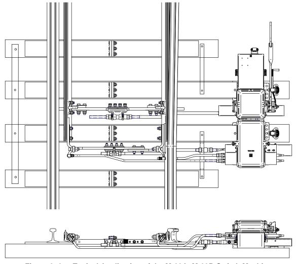
Figure 3-2 - Typical Application of the M-23A, M-23B Switch Machine
