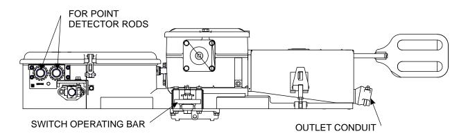
Figure 1-2 - Outline Diagram of the M-23A, M-23B Switch Machines
