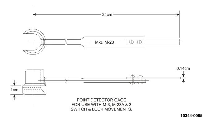
Figure 5–5 - Point Detector Gage N295326
