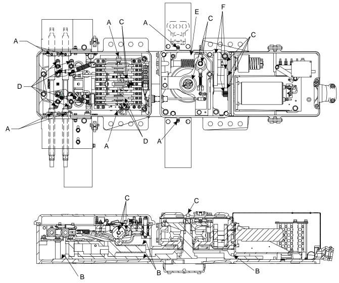
Figure 5-3 - Lubrication Diagram for M-3 Switch Machine
