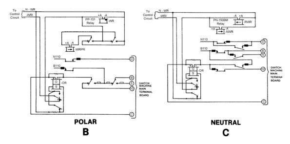
NOTE: EXTERNAL CONNECTIONS ARE SHOWN TO THE MAIN TERMINAL BOARD FOR A SWITCH HAVING THE RIGHT-HAND POINT NORMALLY CLOSED.
