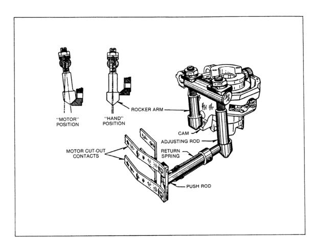
Figure 2–15 - Motor Cutout Contact Assembly (M-23A and M-23B Machines)
