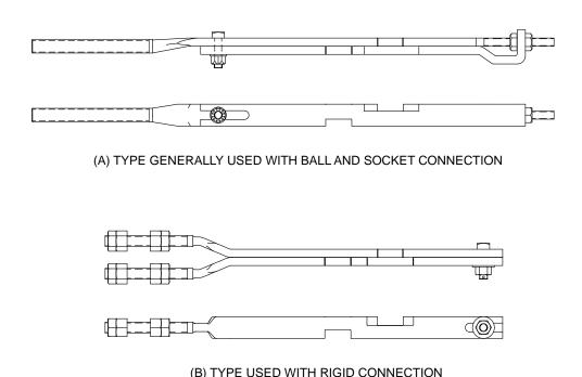
Figure 2-4 - Adjustable Lock Rods for R.H. and L.H. Operation
