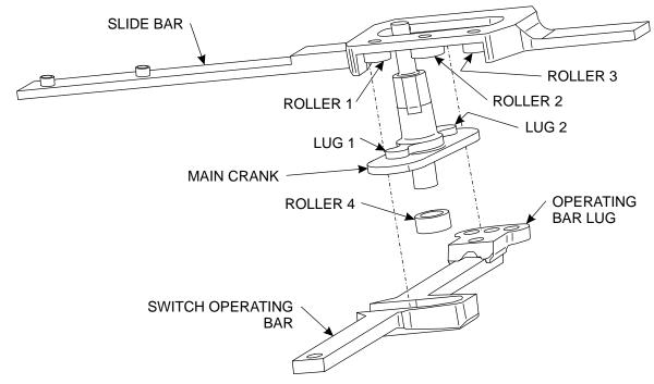
Figure 2–2 - M-3 Switch Operating Mechanism
