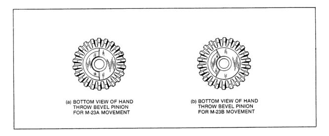
Figure 2-16 - Hand-Throw Bevel Pinions for M-23A and M-23B Switch Machines
