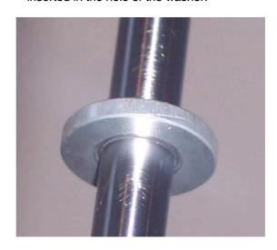
D) Insert the spring guide tube (original BMW)
