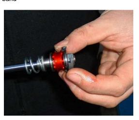
9) Now insert the rod (with its hydraulic piston group) into the cartridge tube
