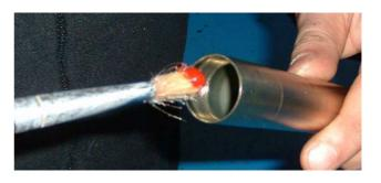
Replace the separator piston O-ring seal. Now insert the separator piston in the cartridge tube, in the correct direction noticed when removed.
