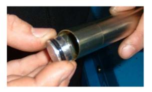
3) Bring on the caliber the measure taken on at the time of removal, therefore push the separator floating piston inside the cartridge up to the wanted distance from the tube edge
