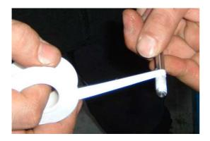
6) Apply on the teflon band the Bitubo grease code 997615
