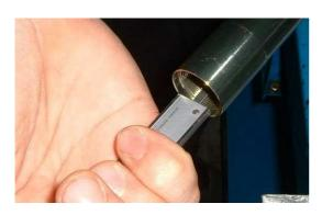
15) Replace the O-ring of the lower cap, and screw it in the tube cartridge
