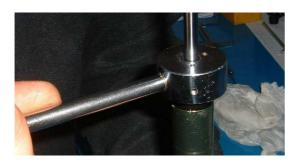
14) verify that the floating piston has not moved during the operations; noticing an inferior measure of 1-2mm respect before these operations, is to consider normal, because due to the tightening of the cap nut on the opposite side.
