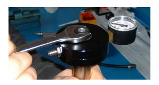
20) Now lock in the wice the lower cap of the cartridge (as shown in photo)
