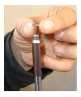
B) Place the RB8 ring in its groove in the rod
