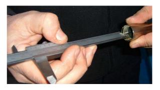
4) Reverse the cartridge, and to pour in the opposed extremity the hydraulic fluid Bitubo code 997631, up to the thread zone
