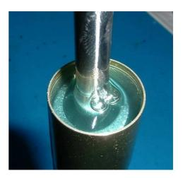
11) To position the washer on the rebound spring
