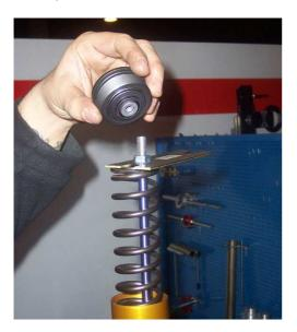
26) With the 13mm wrench (on the rod nut) and the 17mm wrench (on the top cap), tighten the nut to lock the top cap
