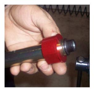
9) Now lock the cartridge in vice, and with the 17 mm wrench slowly unscrew the lower closing cap, for depressurize the cartridge
