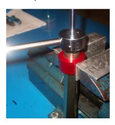
13) Unscrew completely the cap nut, and pull it upward along rod pumping
