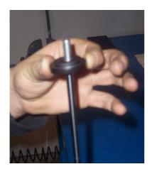
8) To hold in the vice the body cartridge, insert it in the Bitubo tool code 00396 as shown in photo
