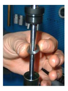
14) Extract the cartridge rod, complete of its hydraulic piston, and remove
