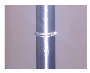
C) Insert in the rod the washer (original spring guide stopper) with the working face down, until the RB8 ring. Verify that the ring is fully inserted in the hole of the washer.
