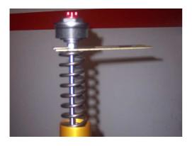
Holding the locking rod nut with the wrench 13 mm, with the wrench 17 mm to unscrew the top cap of the fork legs
