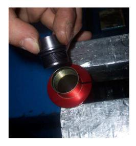
11) Measure and take note the distance of the oil/gas separator floating piston from the edge of the cartridge
