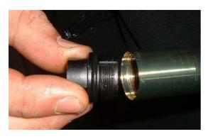
16) Screw the lower cap until the distance of 1-2 mm from the O-ring (see photo), to allow the insertion of gas with the Bitubo special tool.
