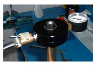
19) Now tighten the cap using the 17mm wrench
