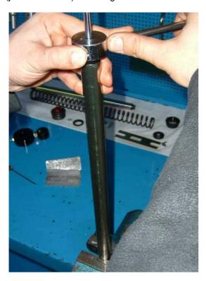
22) insert the lower spring plate, in the righ position (shape upward)
