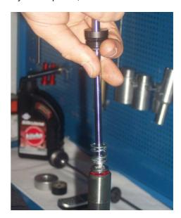
15) Remove from the hydraulic piston the sliding band
