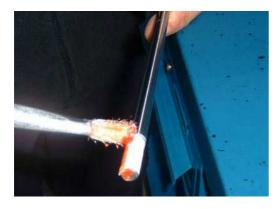
7) Insert in the rod the washer (of the rebound spring), and then insert in the rod the new nut cap complete of new O-ring and rod oil seals (included in Kit Revision Ref. GR0074)
