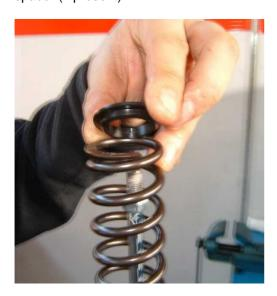
25) Compress the spring, and insert under the nut the Bitubo tool cod. 00317, then screw the top fork cap
