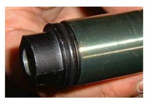
17) Apply on the cartridge tube (as shown in photo) the Bitubo insertion gas tool cod. 00231 (Ø 25 mms)
