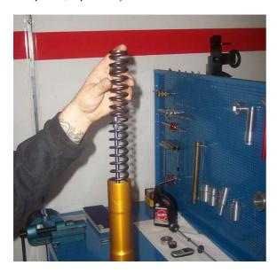
6) Unscrew and remove the locking nut of the rod
