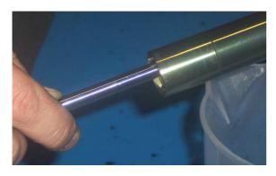
18) So this will make it possible to go out the floating piston to the opposite extremity of the tube cartridge.
