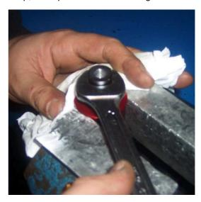
10) Unscrew completely, and remove the cap
