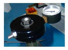
18) Insert the Nitrogen gas at pressure of 8.0 bar
