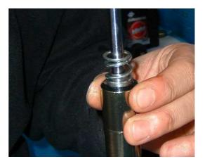
10) Push the rod until the rebound spring arrives at the end of the threaded zone
