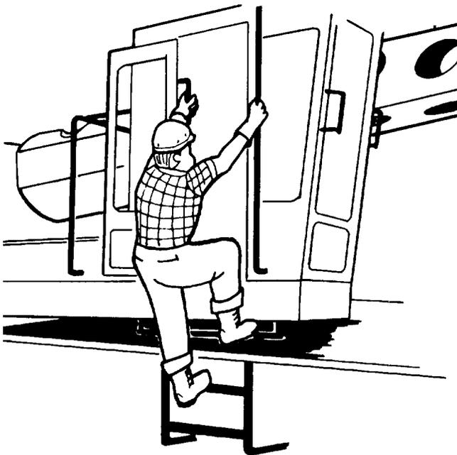
**Maintain three point contact** with grab handles and steps when climbing on and off the machine. **Never jump from the machine.**
