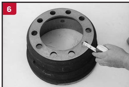
Number, size, and location of bolt holes
