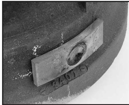
Welded balance weight
