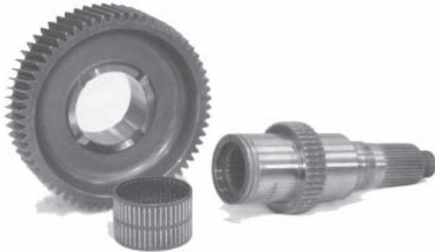
26. Remove 1st gear and the bearing from the shaft. The clutch gear is a part of the shaft.
