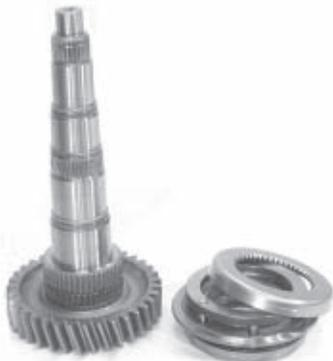
9. Remove the 2nd/3rd speed synchronizer.
