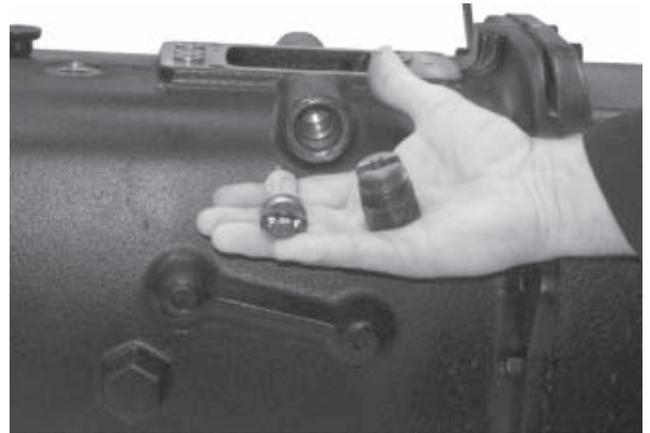
5. If the driver has experienced shifting problems, check the crossgate plunger and spring at this time. Replace them if they are worn or damaged. If no problems have occurred, it is not necessary to remove the plunger.
