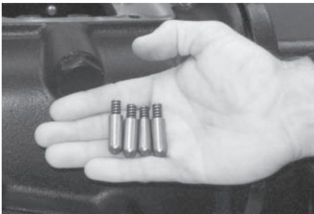
3. The four springs and plungers should be removed now. If the reason for the teardown was a shifting problem, closely examine the springs and plungers for wear or damage. Replace them if they are worn or damaged.
