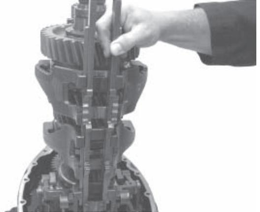
4. Remove rail channel from shift forks and front bar support.
