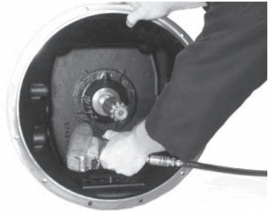
11. Next, tip the clutch housing up. Remove the four drive gear bearing cap capscrews.
