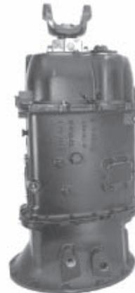
18. Install the flange or yoke. Secure with a nut. Torque to 300 - 325 ft. lbs.
