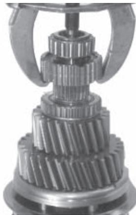
3. Attach a puller to the 6th/7th speed clutch gear. Remove the gear and the drive gear bearing together.
