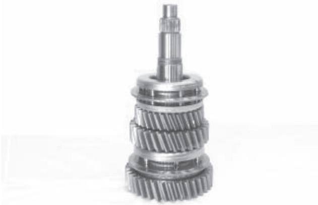
7. Lubricate then Install the 4th/5th speed synchronizer.
