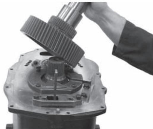
6. Use Moly #2 lubricant to coat the mainshaft splines. Then install the rear mainshaft.
