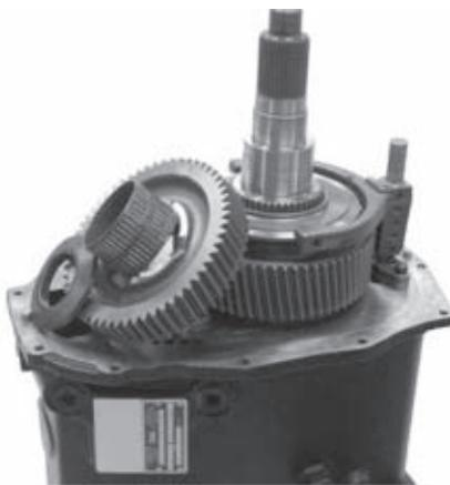
9. Next install the caged bearing and reverse gear. The gear hub should face the bearing. Also install the thrust washer, with the tapered side up.
