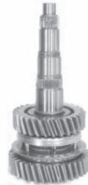
4. Place the caged needle bearing and 3rd speed gear onto the shaft. The gear hub should point toward 2nd/3rd speed synchronizer. Position the lock ball into the shaft and slide the thrust washer into place.
