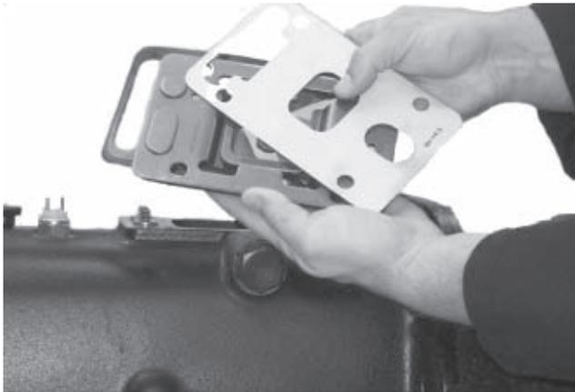
2. Remove the interlock retaining drive screws. Next remove the gaskets and interlock retainer plate.
