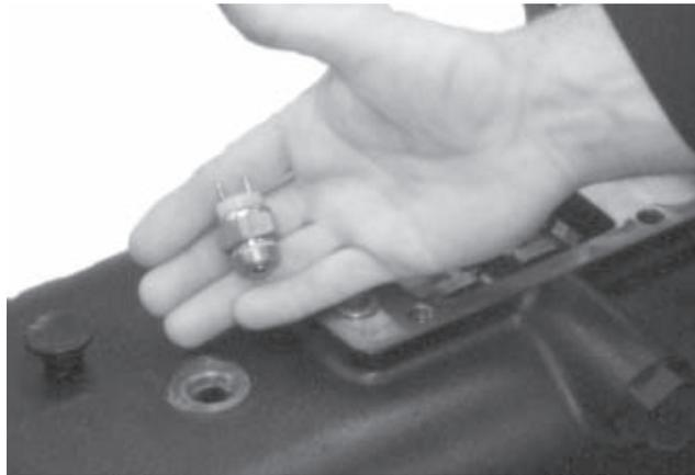
20. Install the backup light switch if it was removed earlier. Torque it to 25 - 41 ft. lbs.
