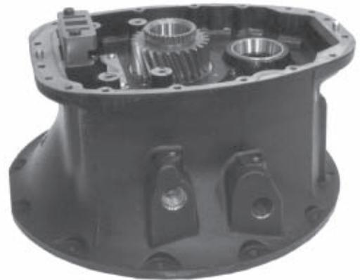
5. Place the clutch housing, drive gear face down, on the workbench.
