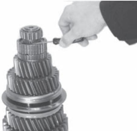
2. Remove the spiral snap ring from the groove. The easiest way to do this is to place a screwdriver under one end and work it around the snap ring.
