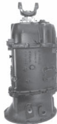
6. Attach a bracket or lift hooks to the rear case. Secure with bolts, which are at least hand-tightened. **Lift the transmission with a hoist**, and set it on end on a workbench that contains a hole for the drive gear.
