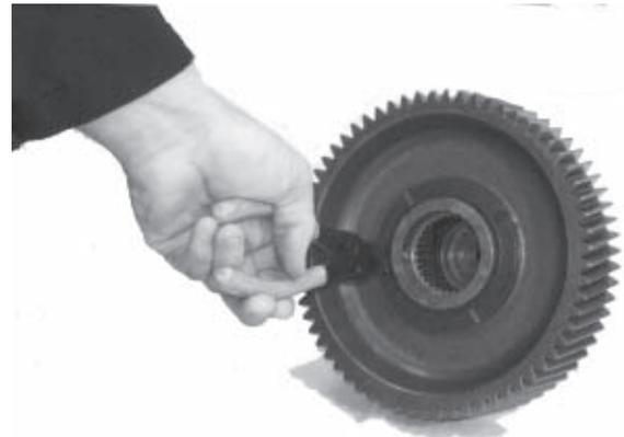
23. To remove 1st gear from the mainshaft, first remove the snap ring. **Always wear safety glasses to protect your eyes when servicing transmissions.**
