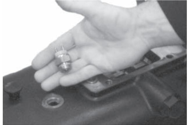
4. The backup light switch can be removed if it is going to be replaced. Otherwise, it does not have to be removed during servicing.
