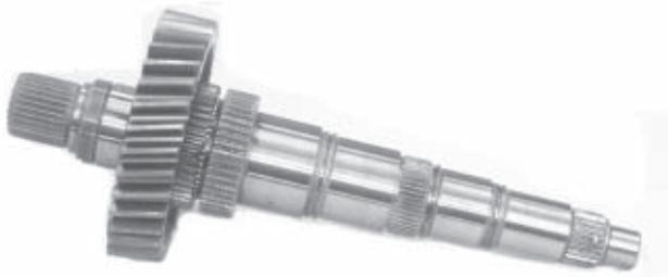
1. Lubricate all bearings with oil before beginning reassembly. Continue by placing the caged needle bearing and 2nd speed gear (hub toward clutch gear) on the shaft. Position the thrust washer on the shaft, then press the bearing race into place.
