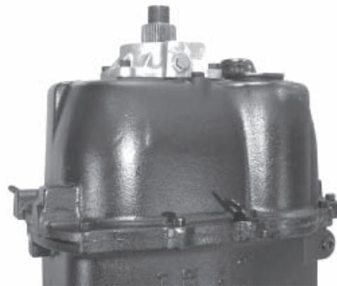
17. Secure the bearing cap with cap screws. Torque them to 25 - 41 ft. lbs.
