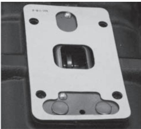
27. Install final gasket and note the position of the interlock plate. This photograph shows the correct position.
