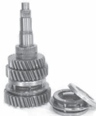
6. Remove the 4th/5th speed synchronizer from the shaft.
