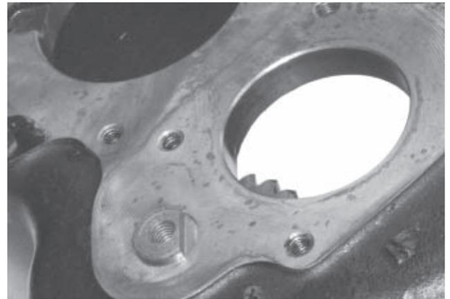
11. The straight edge on the end of the idler shaft must be positioned as shown here. Tap it into the case so the top portion of the shaft is flush with the case, or not more than .030" below the case surface. The lower portion of the idler shaft will extend about 1/4" above the case.
