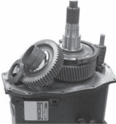
20. Continue by removing the thrust washer, reverse gear, and the caged needle bearings.
