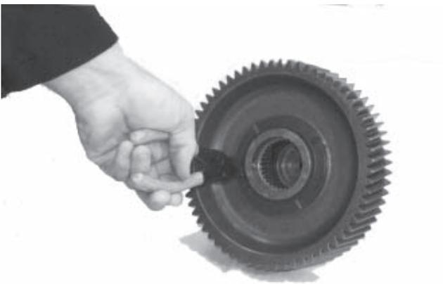
3. Next install the bearing and 1st gear onto the rear mainshaft. **Also install the lock ball, thrust washer, and snap ring.**
