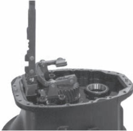
7. The overdrive fork is pictured here. It is not necessary to remove this fork, although the technician may wish to do so.
