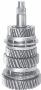
8. Next, install the two caged needle bearings and 5th speed gear. The gear hub should face the synchronizer. Put the lock ball into place. **Then install the thrust washer and snap ring.**
