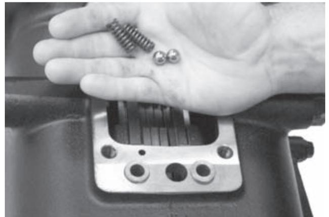
23. Install detent ball and detent springs.
