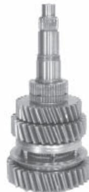
6. Continue by placing two caged needle bearings (wider one first) on the shaft. Slide 4th speed gear on the shaft with the clutching teeth up. Also install 4th/5th speed clutch gear. **Secure it with a snap ring.** The rounded side of the snap ring should face the clutch gear.
