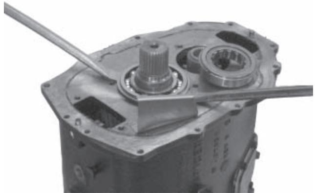
28. Use pry bars to remove the mainshaft and countershaft bearings.
