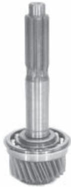
1. **Press the bearing into place and install snap ring.** Then use a suitable press to push the oil ring into place. A brass hammer can also be used for this procedure.
