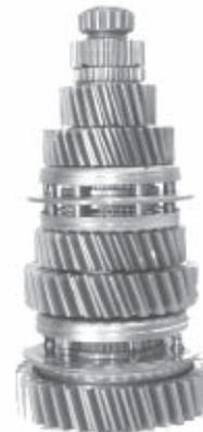
10. **Press the bearing onto the end of the shaft.** The chamfered side of the bearing should face the 6th/7th speed clutch gear.
