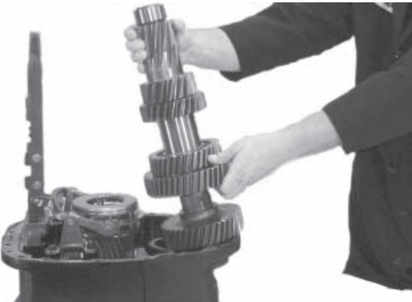
8. The countershaft is installed next. Tilting the countershaft toward the mainshaft is the easiest way to do this. Notice that there aren't any timing marks on the gears. There is no need to time the countershaft to the mainshaft.
