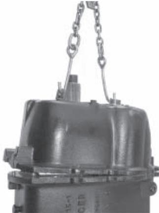
14. Then use a chain hoist to remove the rear housing.
