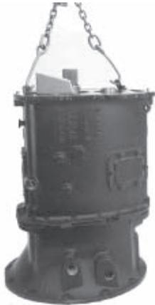
2. Begin main case disassembly by removing the housing.
