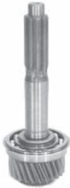
1. **Press the bearing into place and install snap ring.** Then use a suitable press to push the oil ring into place. A brass hammer can also be used for this procedure.
