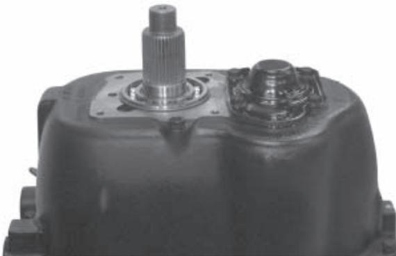
14. Secure the cap with cap screws. Torque them to 25 - 41 ft. lbs.
