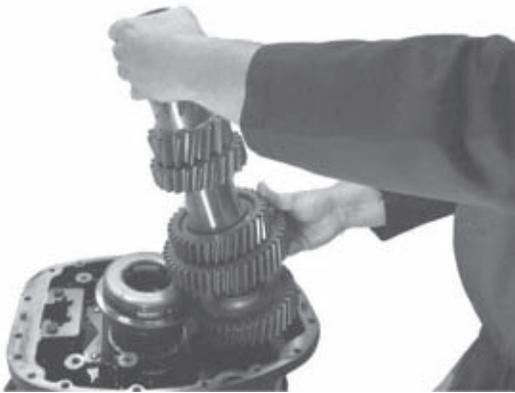
8. Remove countershaft (tilting the countershaft is the easiest way to do this).
