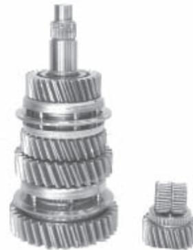
4. Next remove the overdrive gear in an overdrive unit, or 6th speed gear in a direct drive unit. There are two caged needle bearings in the gear.
