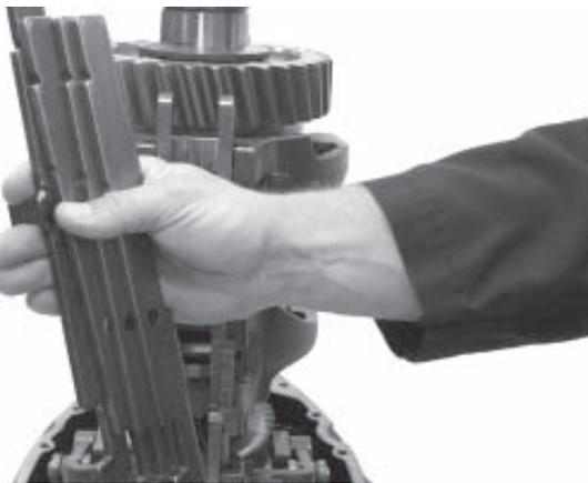
3. Remove shift rails from rail channel.
