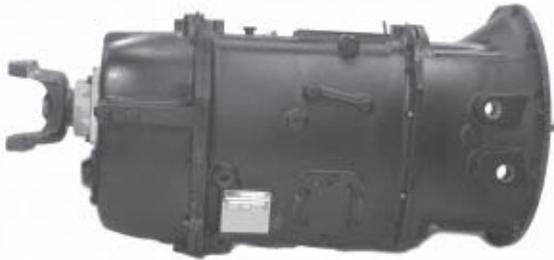
1. After removing the transmission from the vehicle, drain the oil. **Let the unit cool down first.** Otherwise, hot transmission fluid could cause burns.
