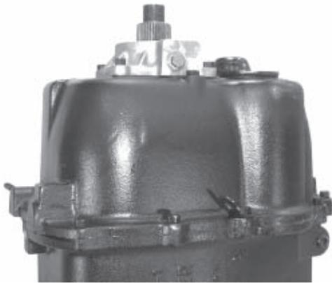
7. Remove the nut, washer, and end yoke or flange.
