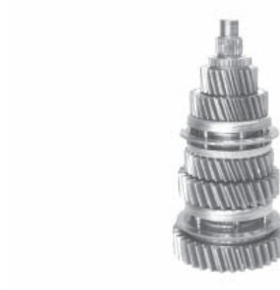
9. Install two caged needle bearings and either the overdrive gear (for the overdrive version) or the 6th speed gear (for the direct version). The clutch teeth should face up. Install the 6th/7th speed clutch gear, and secure it with the spiral snap ring.
