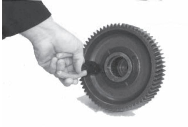
5. Next install the bearing and 1st gear onto the rear mainshaft. **Also install the lock ball, thrust washer, and snap ring.**
