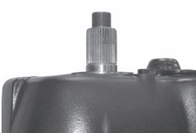
9. Next remove the speedometer signal gear.
