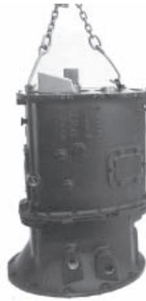
11. Coat the clutch housing sealing surface with purple Loctite 515 or the equivalent. **Lower the case into place with the help of a chain hoist.** Secure it with bolts. Torque to 25 - 41 ft. lbs.
