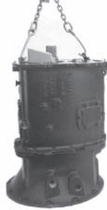
14. Coat the clutch housing sealing surface with purple Loctite 515, or equivalent. **Lower the case into place with the help of a chain hoist.** Secure it with bolts. Torque to 25 -41 ft. lbs.
