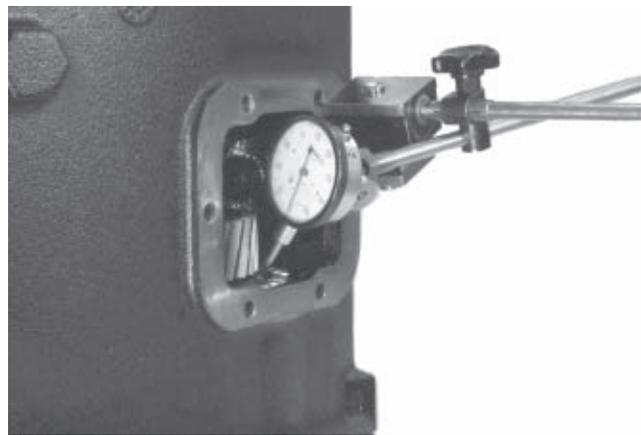
18. Remove the PTO cover and position a dial indicator as shown. Use a pry bar to lift up on a gear. End play should measure between .001"-.008". If end play is correct, replace the PTO cap and torque the cap screws to 25 - 41 ft. lbs. If end play is not correct, add or subtract shims under the rear countershaft bearing cap.
