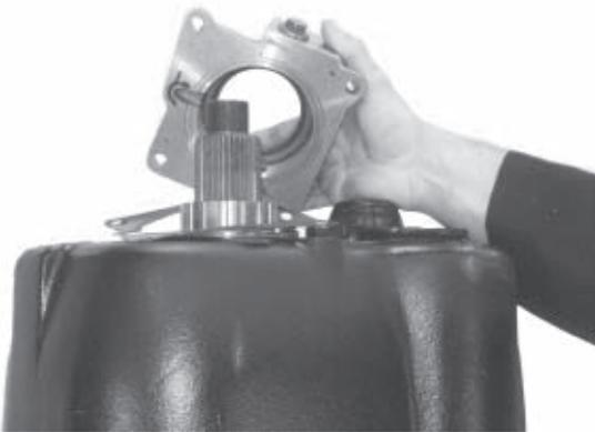
8. Remove the output bearing cap and gasket.
