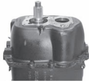
11. Coat the case sealing surface with purple Loctite 515 or the equivalent. **Then install the rear case with the aid of a chain hoist.** Secure with capscrews. Torque them to 25 - 41 ft. lbs. If a new 1st/reverse shift bar support was installed in the rear case, make sure the 1st/reverse bar is shifting properly.
