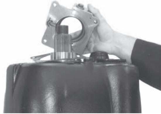
16. Install the signal gear and the mainshaft bearing cap and gasket. Make sure the bearing cap oil passage lines up with the oil passage in the transmission housing.
