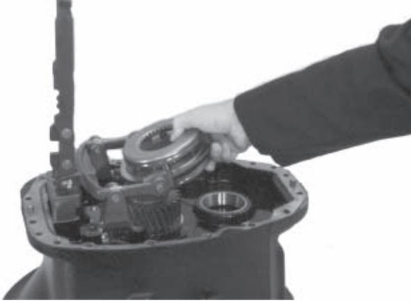
7. Next lubricate then install the 6th/7th speed synchronizer. Shift it down toward the drive gear. This will aid alignment.
