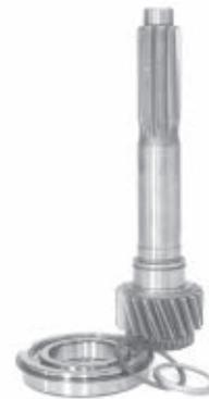
14. Continue by removing the snap ring and oil ring. Also remove the bearing.
