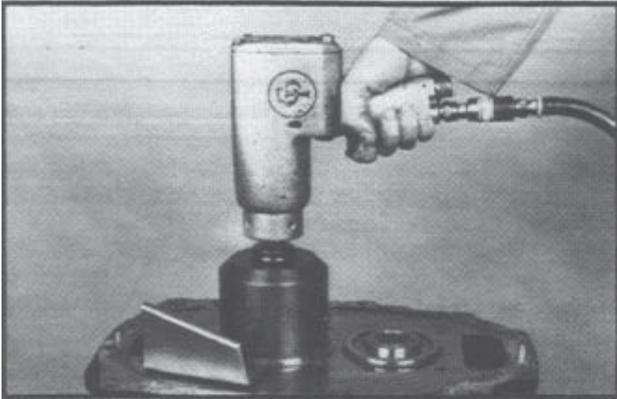
This Spicer transmission can be repaired with ordinary mechanic's tools. However, if your transmission has a mainshaft intermediate nut rather than a snap ring, vehicle downtime can be minimized with the use of this special socket. It is available through Sealed Power Corporation, part number OEM6599. To order, contact:
