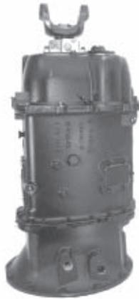
19. Install the flange or yoke. Secure with a nut. Torque to 300 - 325 ft. lbs.
