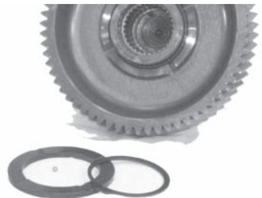
24. Remove the thrust washer and lock ball next.
