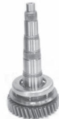
3. Lubricate the 2nd/3rd speed synchronizer with oil, then slide it onto the shaft. Shift it into 2nd gear.
