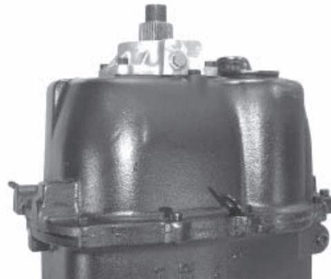
16. Secure the bearing cap with cap screws. Torque them to 25 - 41 ft. lbs.
