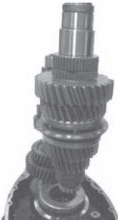
8. Oil the pocket bearing race, then slide the mainshaft assembly into place. It may be necessary to tip the countershaft away from the mainshaft to do this.
