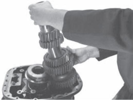
7. The countershaft is installed next. Tilting the countershaft toward the mainshaft is the easiest way to do this. Notice that there aren't any timing marks on the gears. There is no need to time the countershaft to the mainshaft.
