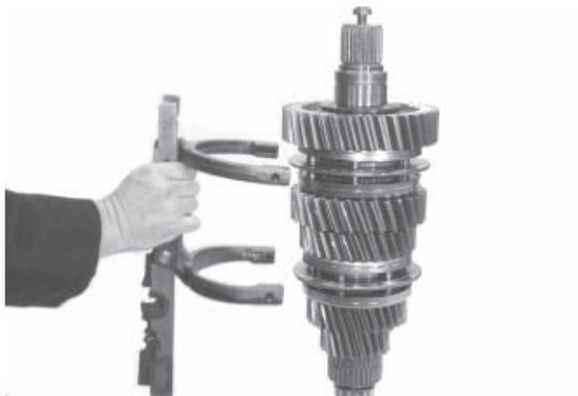
9. **Lift the mainshaft with a hoist.** While it is in the air, install 2nd/3rd and 4th/5th speed forks into place.
