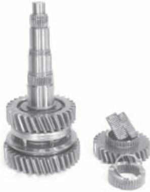
7. **Wearing safety glasses, remove the snap ring and 4th/5th speed clutch gear.** Also remove 4th speed gear and the two caged needle bearings. Notice that one bearing is wider than the other. This will be important during reassembly.
