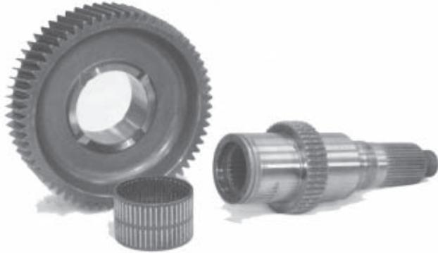
25. Remove 1st gear and the bearing from the shaft. The clutch gear is a part of the shaft.
