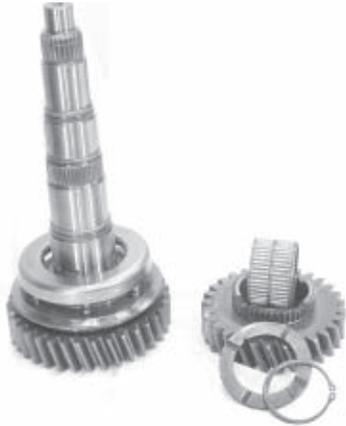
8. **The snap ring, thrust washer, and lock ball can be removed.** Also remove 3rd speed gear and the caged needle bearing.
