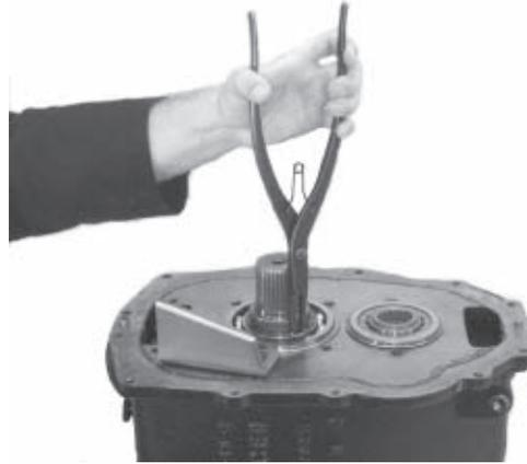
27. Lock the transmission into two gears. Remove the snap ring or mainshaft intermediate nut, depending on which component your unit contains. If your unit contains the mainshaft intermediate nut, the easiest way to remove it is to use the special socket pictured on the tool reference page.
