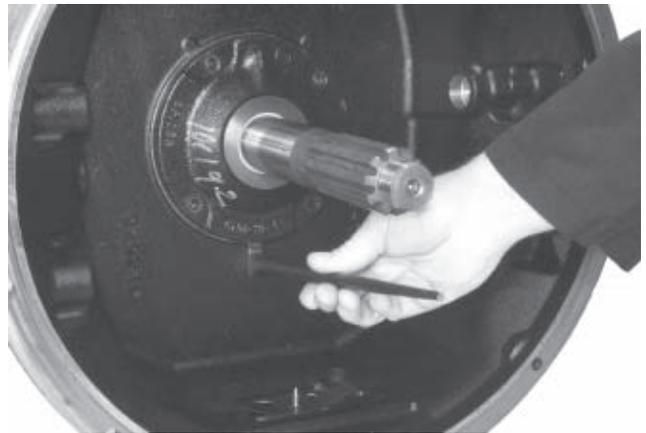
12. Use the milled slot to pry the bearing cap away from the housing.
