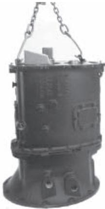
2. Begin main case disassembly by removing the housing.
