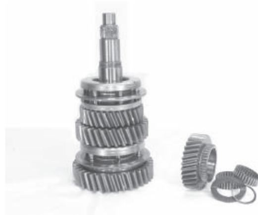
5. Remove the snap ring, thrust washer, and lock ball. (The lock ball prevents the thrust washer from turning on the shaft.) Also remove 5th speed gear, and the two caged needle bearings.
