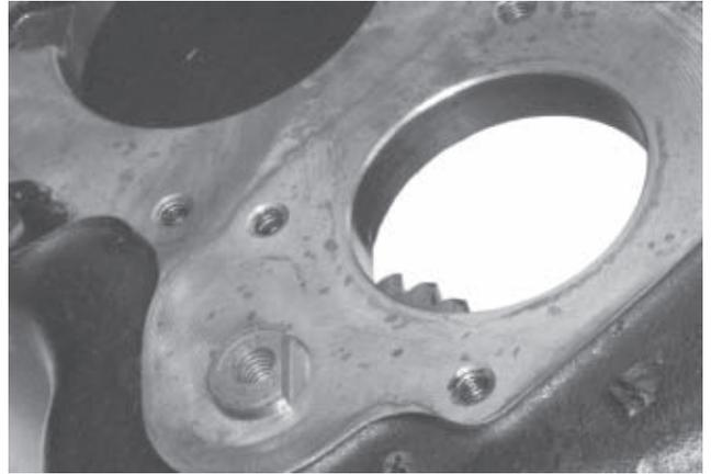
10. The straight edge on the end of the idler shaft must be positioned as shown here. Tap it into the case so the top portion of the shaft is flush with the case, or not more than .030" below the case surface. The lower portion of the idler shaft will extend about 1/4" above the case.
