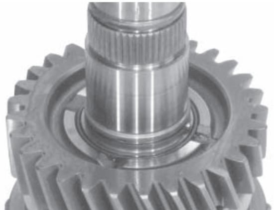
5. Note that the lock ball keeps the thrust washer from rotating on the shaft. **Wearing safety glasses,** Continue by installing the snap ring with the rounded side toward the thrust washer.
