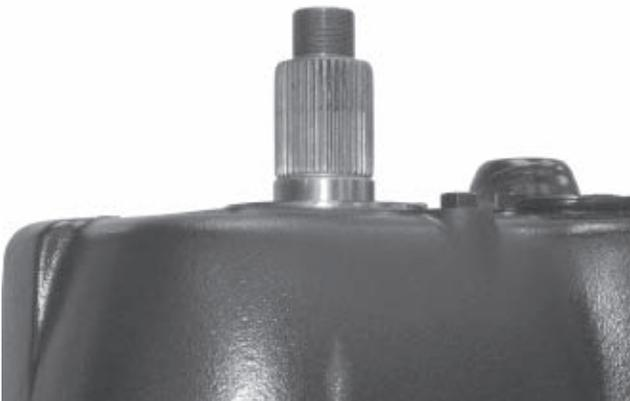
9. Next remove the speedometer signal gear.
