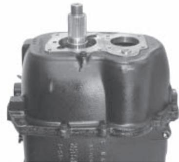
12. Coat the case sealing surface with purple Loctite 515 or the equivalent. **Then install the rear case with the aid of a chain hoist.** Secure with cap screws. Torque them to 25 - 41 ft. lbs. If a new 1st/reverse shift bar support was installed in the rear case, make sure the 1st/reverse bar is shifting properly.
