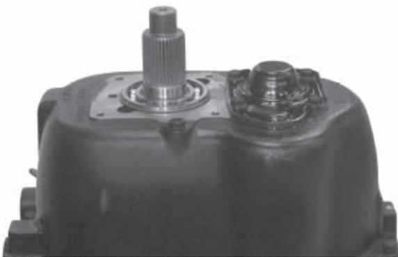
15. Secure the cap with cap screws. Torque them to 25 - 41 ft. lbs.
