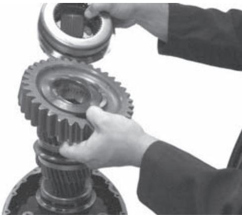
9. Lubricate the 2nd/3rd synchronizer with oil, then slide it onto the shaft. Continue by placing the caged needle bearing and 2nd speed gear (hub toward synchronizer) on the shaft. Position the thrust washer on the shaft.
