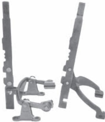
8. The direct shift fork, shown at left, also could be removed at this time.
