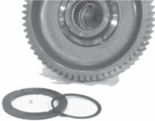
25. Remove the thrust washer and lock ball next.
