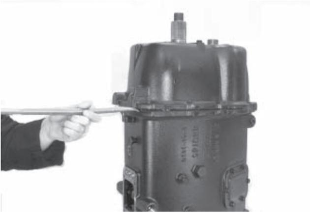
13. Next, place pry bars in the slots provided in the rear case. Break the seal.
